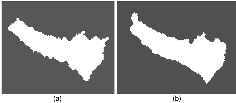
Figure 5-7 Water surface detected in (a) fine resolution and in (b) intermediate resolution
