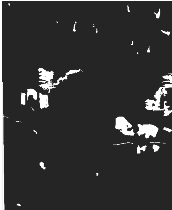
Figure 5-4 Probable water bodies in intermediate resolution after removing the false detections using SVM classification
