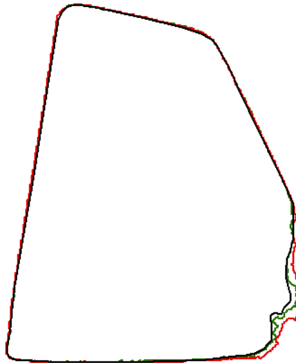
Figure 4-20 Water body detected with MLC (green line), without MLC (red line) and manually drawn breakline (black line)
