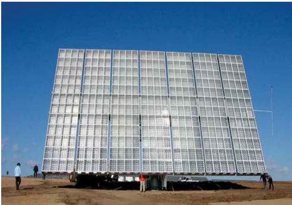
Figure 2.5 Concentrated Photovoltaic (CPV) system
