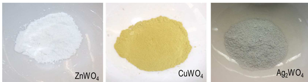
Figure 4-13 Photographs of the SCS tungstate samples using \text{Na}_2\text{WO}_4 .
