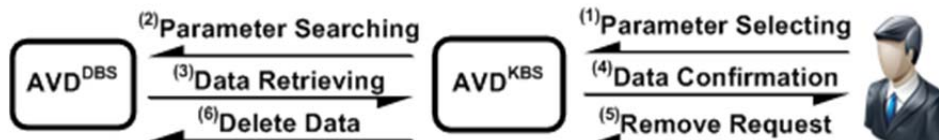
Figure. 4-25 Working Principle of Data Deleting
