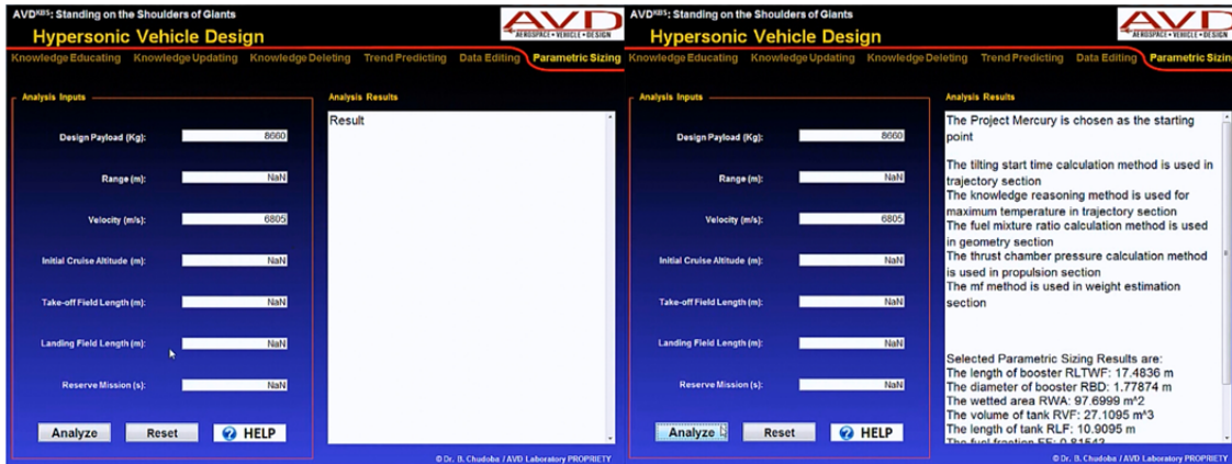
(a) (b) Figure 6-16 (a) Input Mission Requirements, (b) Parametric Sizing Analysis Results
