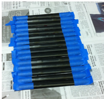
Figure 6-41 Gauge Area Isolated for Paint Spray
