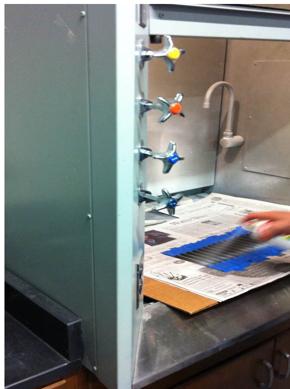
Figure 6-43 Spray Process Conducted inside an Exhaust Chamber
