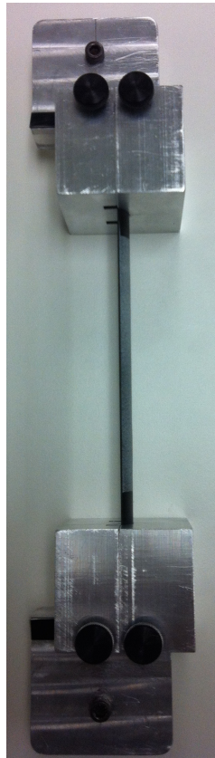
Figure 6-25 Loading Axis Shifted to a Negative Offset from Specimen Edge
