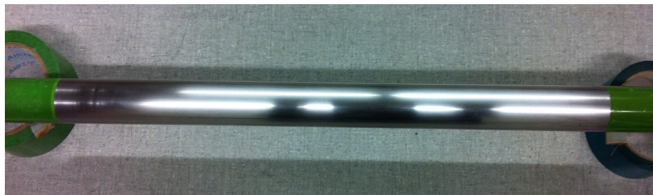
Figure 6-2 Prepped Stainless Steel Mandrel
