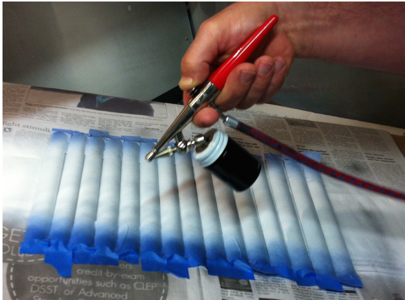
Figure 6-42 Spray Gun Utilized to Generate Uniform Paint Smear
