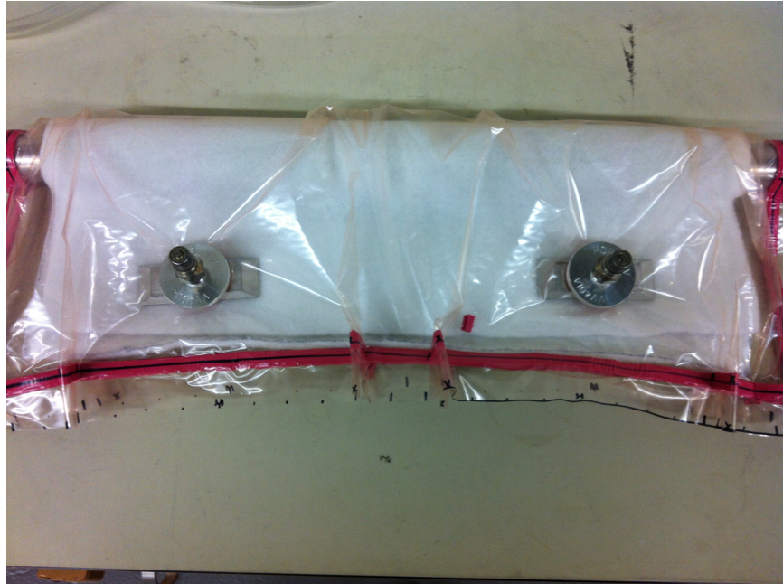
Figure 6-10 Fully Sealed Vacuum Bag Configuration
