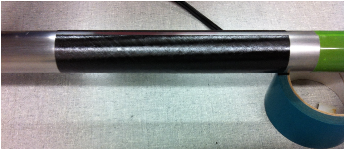
Figure 6-7 Uniform Ply Alignment and Adherence to Mandrel Surface
