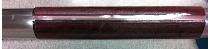
Figure 6-8 Bleeder Fabric applied on Top of Ply Collations
