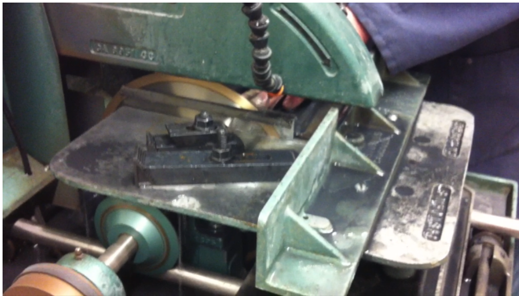
Figure 6-16 Uniform Specimen Slicing by a Composite Saw
