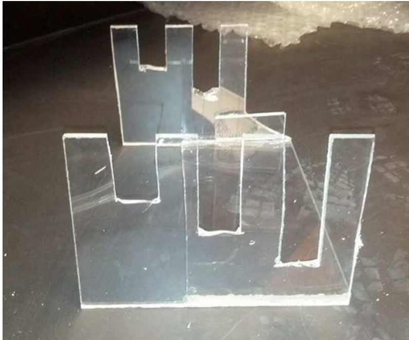
Figure 5-2 Arrangement to hold rebars in oil tank to simulate concrete cover
