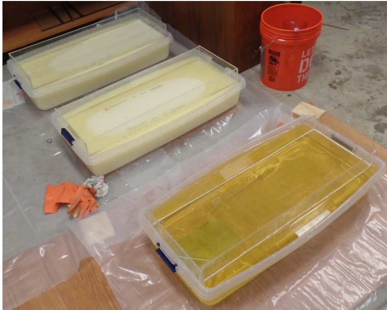
Figure 5-18 Oil emulsion tanks for corroded rebar
