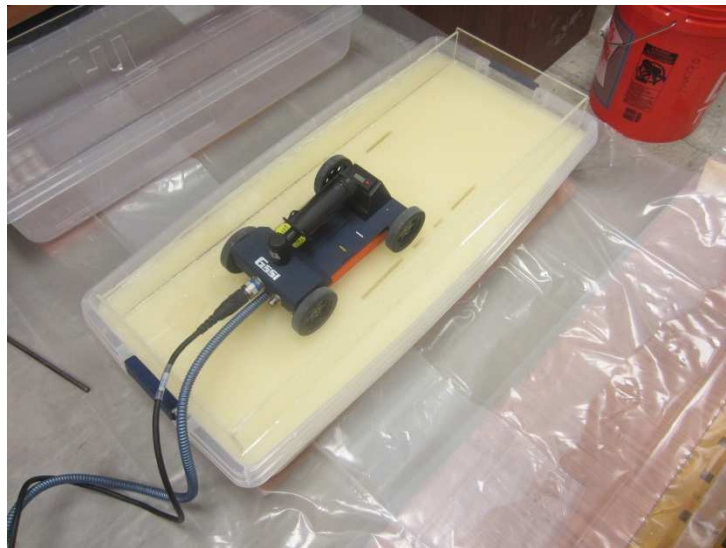
Figure 5-3 Oil water emulsion tank
