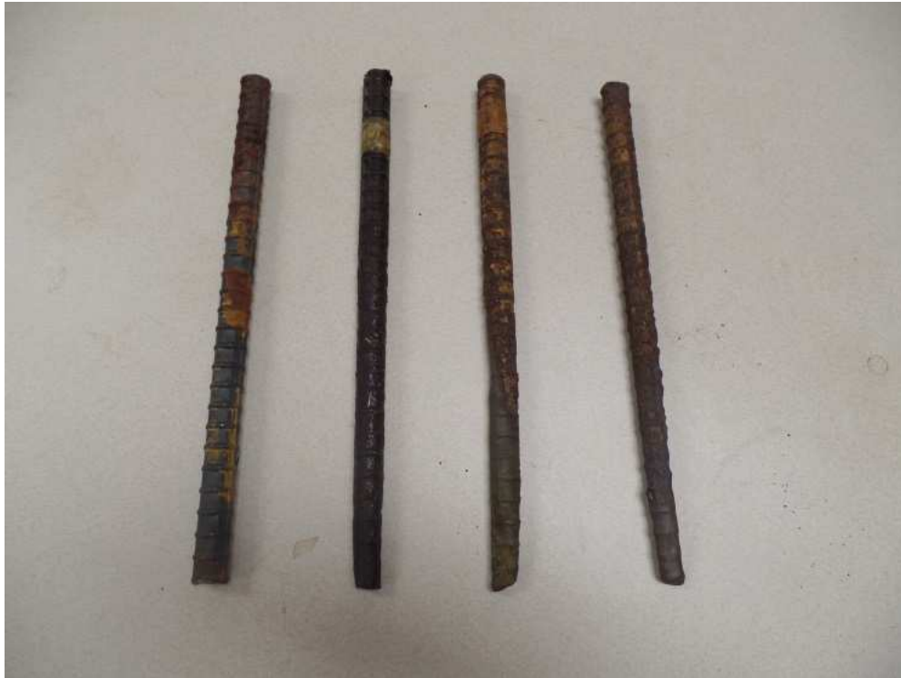
Figure 5-17 Three corroded rebars with a non-corroded rebar on the left
