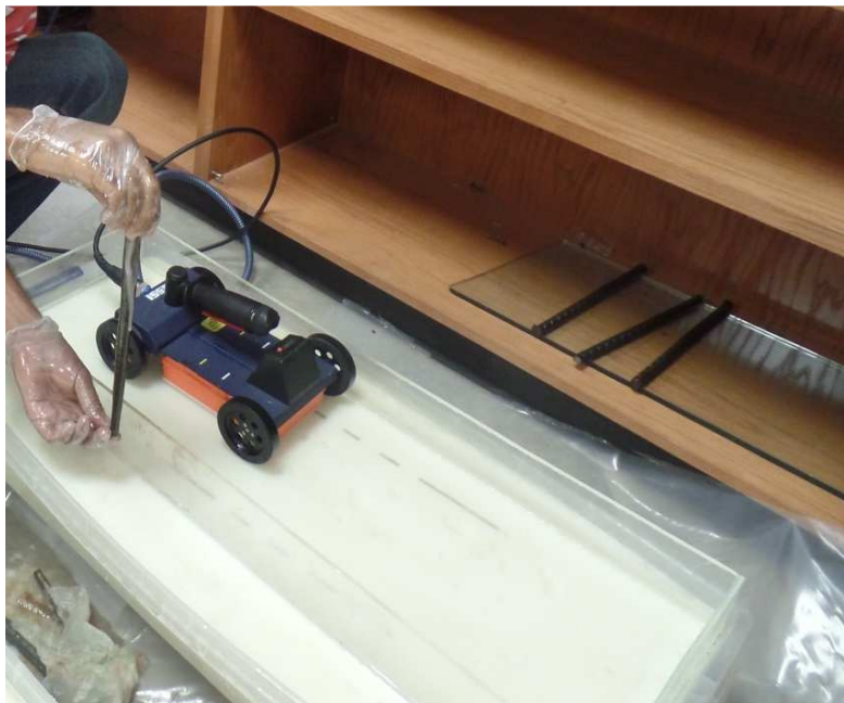
Figure 5-19 GPR Data collection from the corroded rebar in oil emulsion tank
