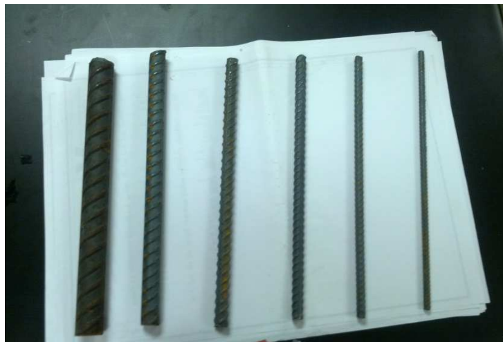
Figure 4-1 Different diameters of the rebar
