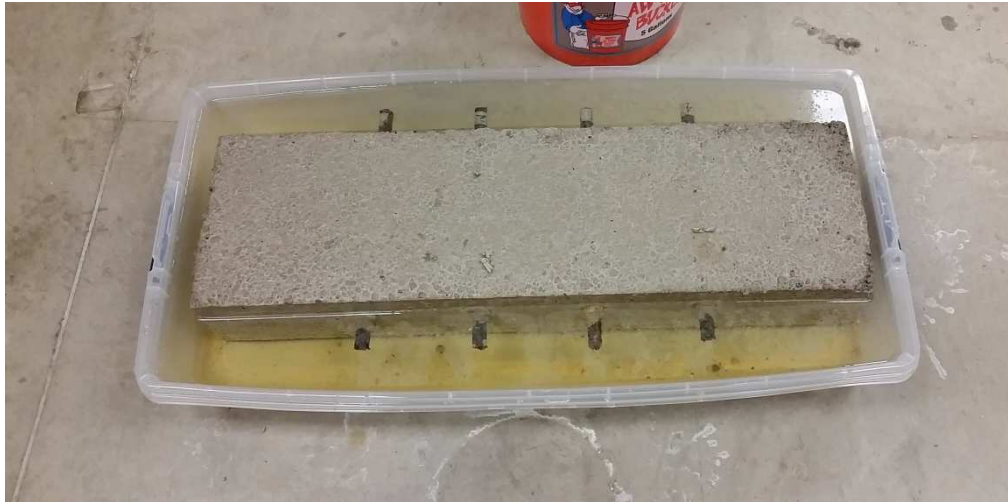
Figure 5-29 Concrete beam with four #5 (16 mm) rebar in 5% salt water solution
