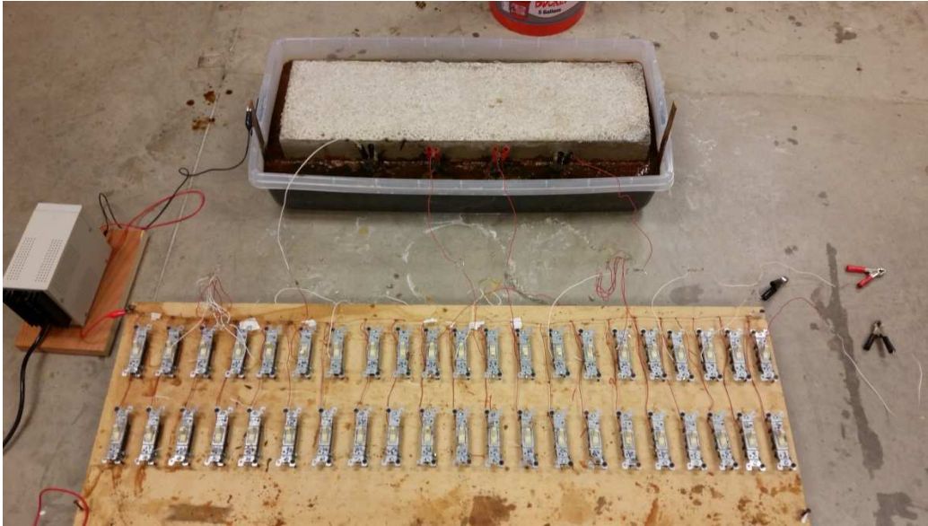
Figure 5-30 Experimental set-up of accelerated corrosion
