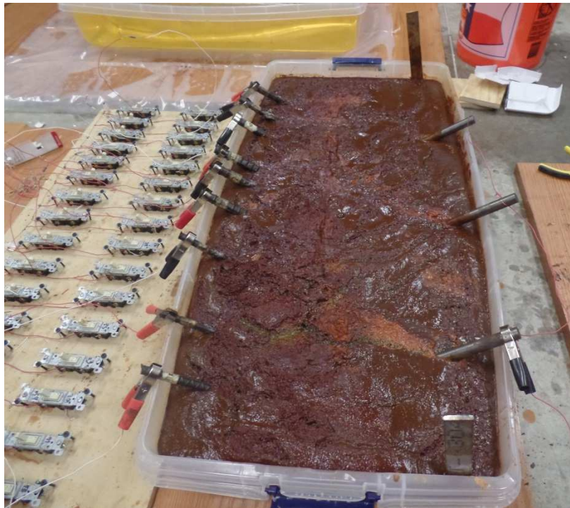
Figure 5-15 Corrosion tank for accelerated corrosion
