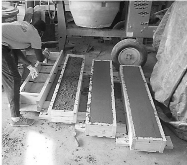
Figure 4-4 Casting of the beam specimens 4.4 GPR scanning and data collection
