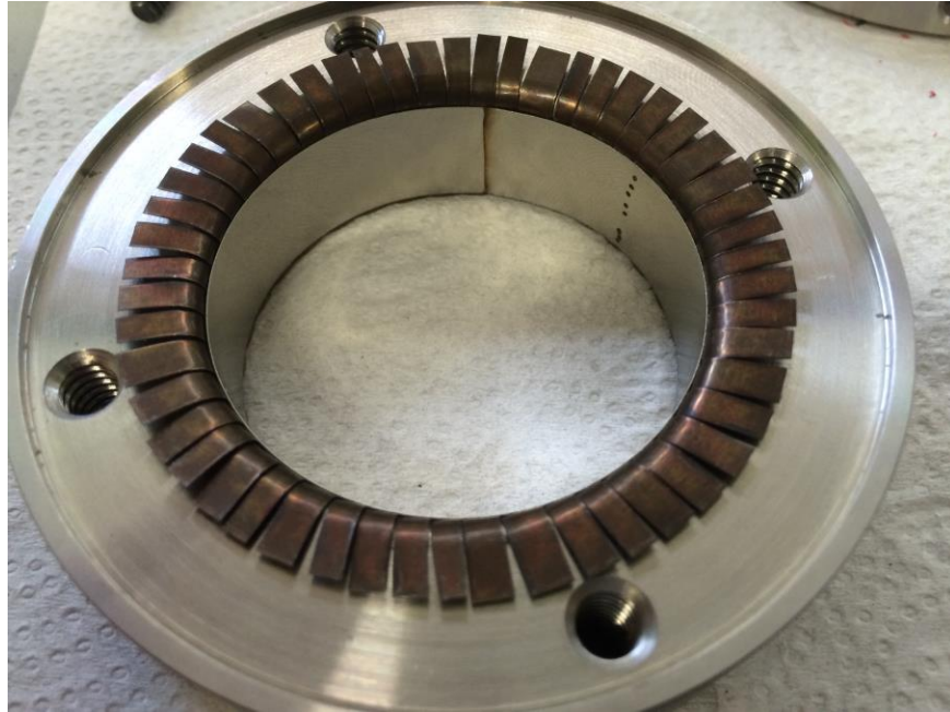
Figure 4-5 One pad foil seal
