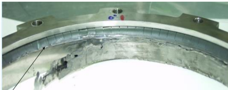
Figure 2-7 Wear of top foil at 30krpm, adopted from Ref [5]
