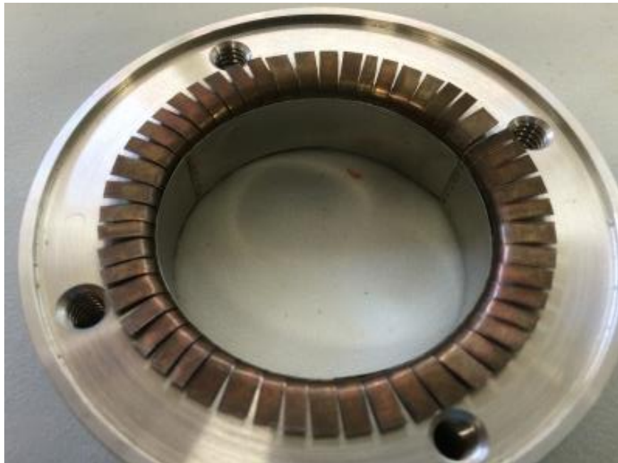
Figure 4-6 Three pad foil seal
