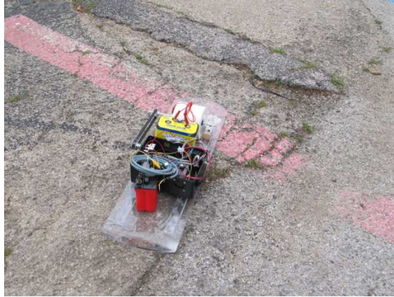
Figure 5-7 Sliding profiler over the rough patch in Tri-C parking lot
