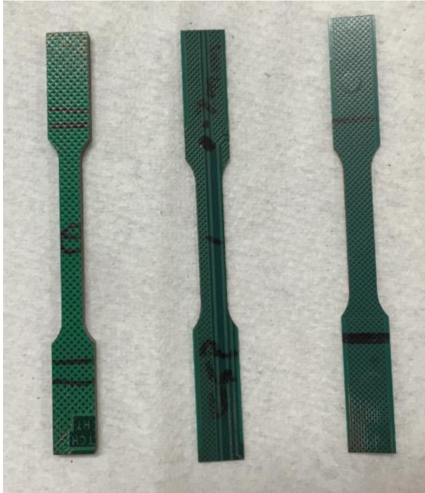
Figure 3.2 Dog Bone Specimen made out of PCB
