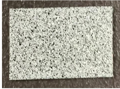
Figure 4.7 Specimen used for measuring the CTE
