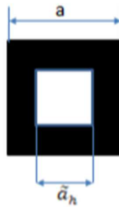
Figure 3-5 Unit cell used in SIMP calculation
