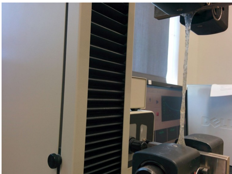
Figure 3.5 Necking in pure polymer during tensile testing
