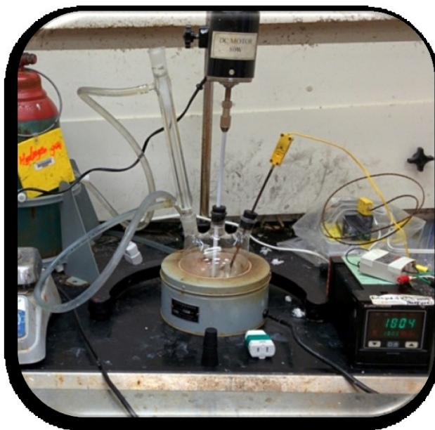
Figure 2.6 Experimental setup for synthesis of the polymer
