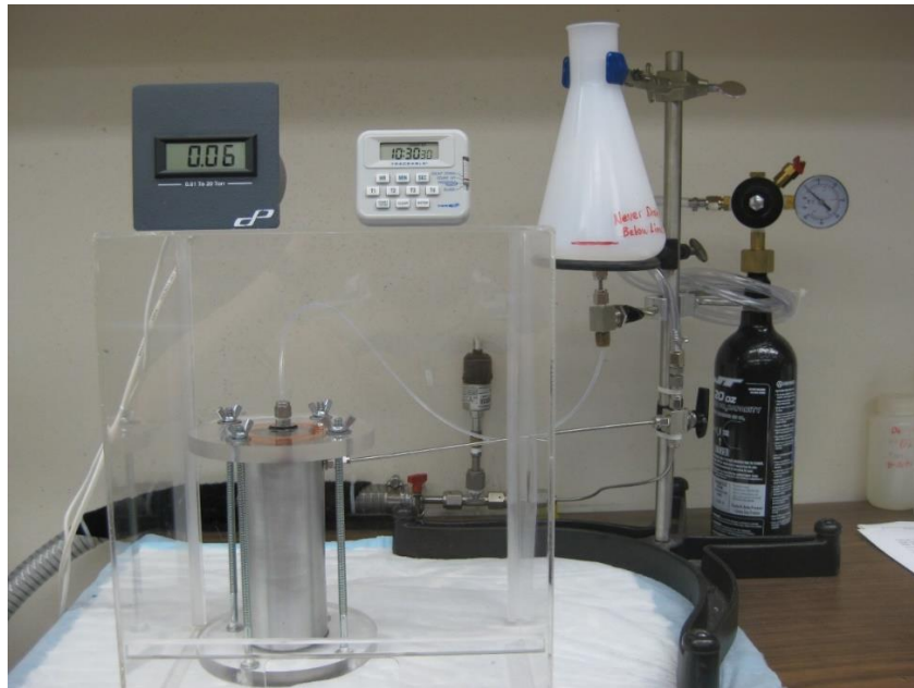
Figure 3-5 Vacuum saturation apparatus.
