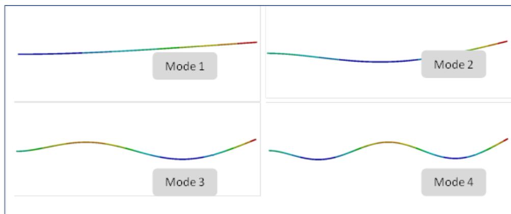
Figure 4-10 FEM results (1D model, 200 NPI) - mode shape, cantilever beam
