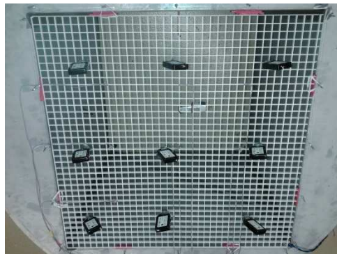
Figure 4.2: RF Code sensors fitted to the mesh setup
