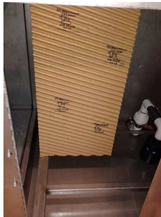
Figure 3.5: Front view of the pad inside the test duct
