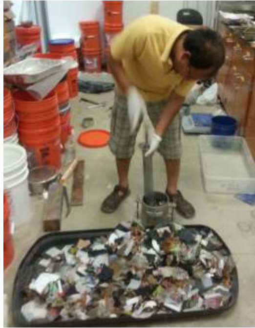
Figure 3-4 Sample compacted for maximum dry unit weight determination
