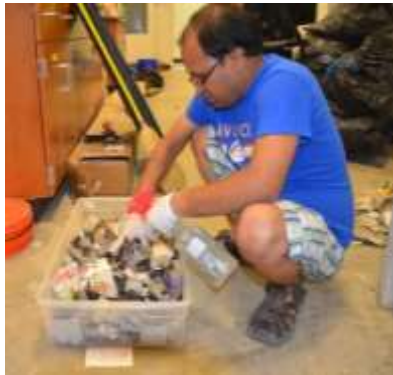
Figure 3-6 Mixing process of shredded waste samples for small and medium permeameter
