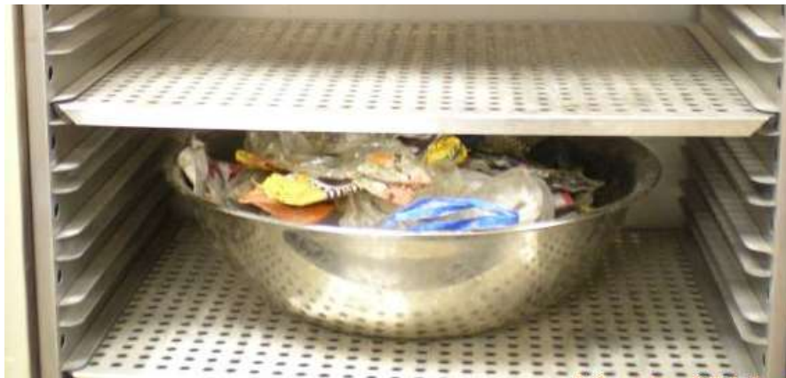
Figure 3-2 Samples placed in oven for determination of moisture content
