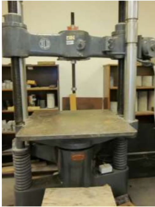
Figure 3-27 Tensile compression machine used for waste compaction
