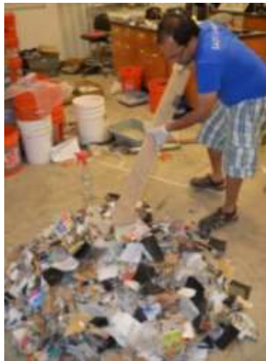
Figure 3-6 Mixing process of shredded waste samples for small and medium permeameter
