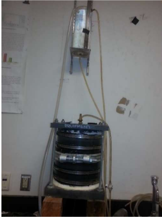
Figure 3-22 Leak-checked test on reactor
