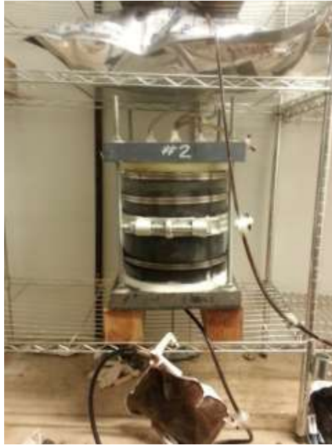
Figure 3-24 A bioreactor cell with different operation systems as leachate collection, gas collection and leachate recirculation
