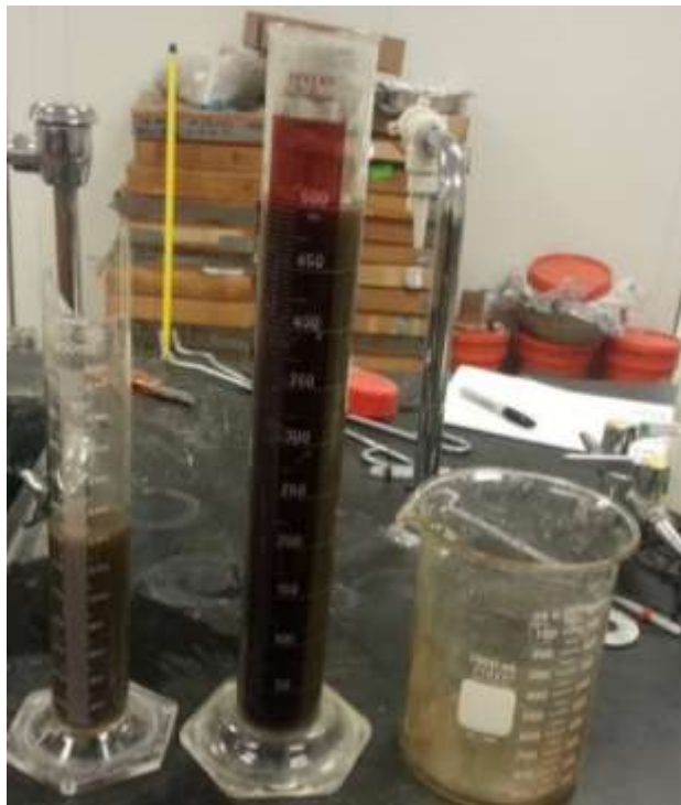
Figure 3-13 Leachate collection and measurement
