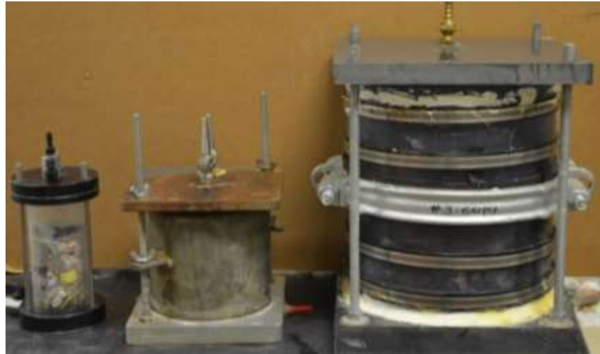
Figure 3-20 Different size permeameters, small-size 6.35 cm; medium-sized 15.24 cm; large-size 25.4 cm diameter (from left to right)
