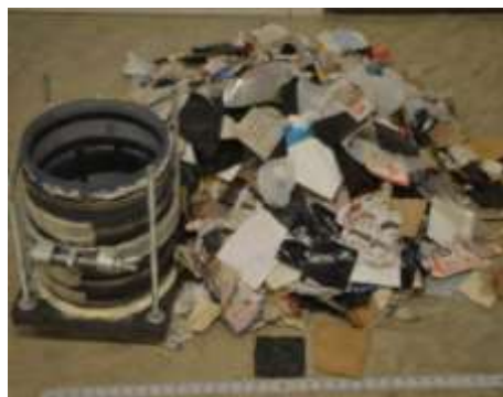
Figure 3-7 Mixing procedure of the shredded waste for large size permeameter
