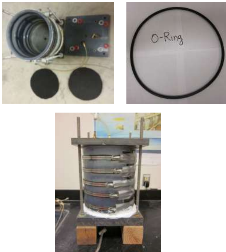
Figure 3-21 Large-size assembled permeameter and its parts
