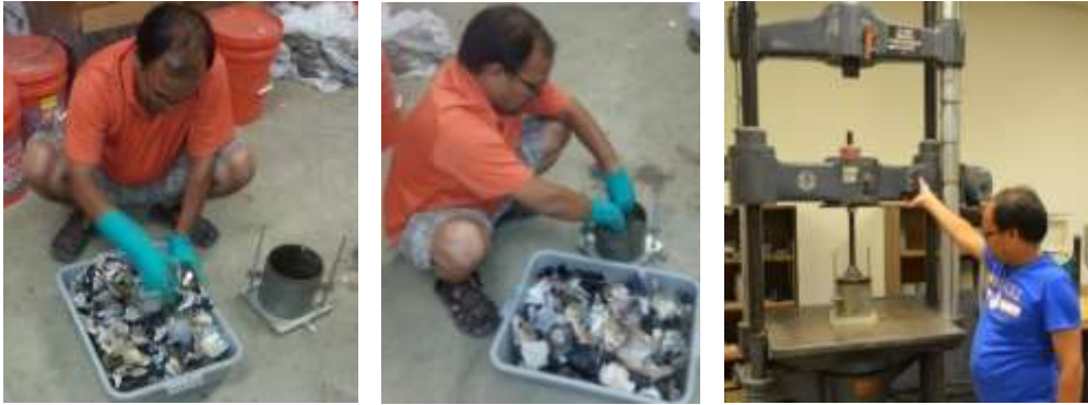
Figure 3-29 Compaction steps of MSW samples on medium 15.24 cm permeameter
