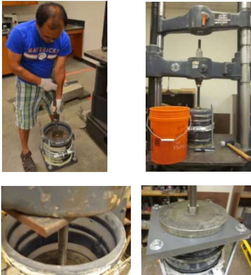
Figure 3-30 Compaction steps of MSW samples in large permeameter and bioreactor cells
