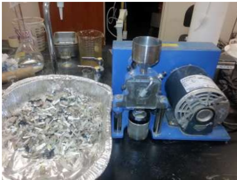
Figure 3-17 Waste grinded in grinding machine for volatile solid test
