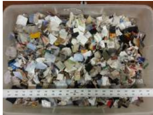
Figure 3-6 Mixing process of shredded waste samples for small and medium permeameter
