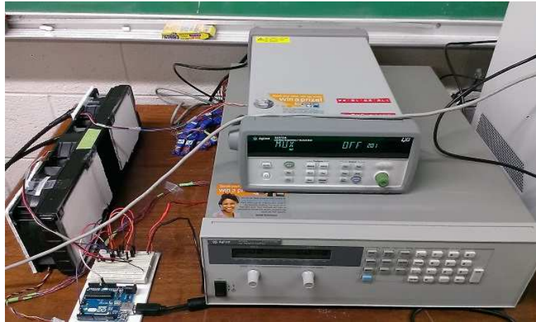
(b) Power Supply (12VDC) to power dry cooler fans
