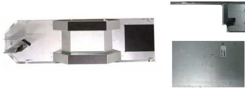
Figure 2.4. Chassis cover with duct.
