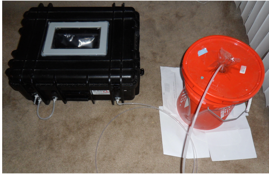
Figure 3.6 Air Sampling by VAC'SCENT Vacuum Chamber
