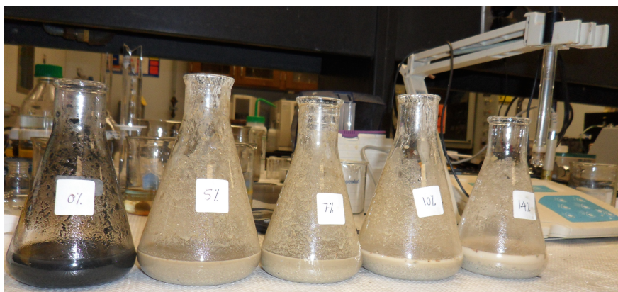
Figure 3.5 Measuring pH of Biosolids with Different Lime Dosages
