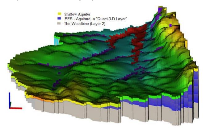
Figure 3-2 Three-dimensional model visualization of the JPL project watershed using USGS Model
