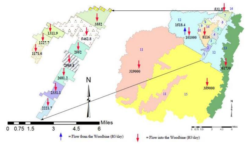
$\textit{Figure 6-8 Distribution of } \underline{\textit{vertical}} \textit{ flow between the Woodbine Aquifer and the shallow groundwater aquifer under pre-lake conditions}. \\$
