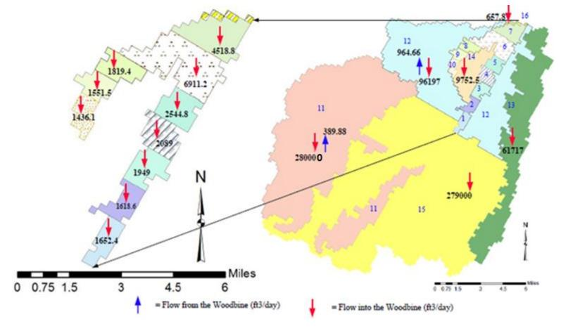
$\textit{Figure 6-7 Distribution of } \underline{\textit{vertical}} \textit{ flow between the Woodbine Aquifer and the shallow groundwater aquifer under post-lake conditions}. \\$
