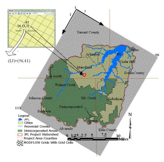
Figure 3-1 Map view of the model mesh. Horizontal array of grid cells used in simulation indicating row (i) and column (j); the horizontal grid size is 1,000 feet X 1,000 feet, but the vertical layer thickness (which is shown in Figures 3-3 and 3-4) is variable in almost all cells
