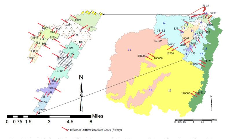
Figure 6-6 The distribution of horizontal flow between zones in the shallow groundwater aquifer under post-lake conditions.
