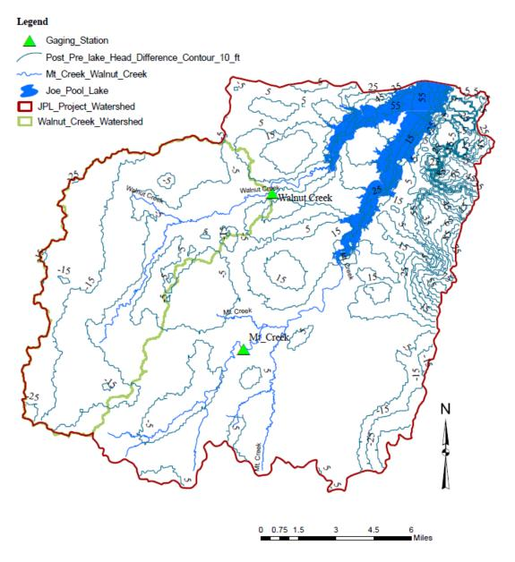
Figure 6-3 The head difference between the post-lake and pre-lake conditions of shallow aquifer
