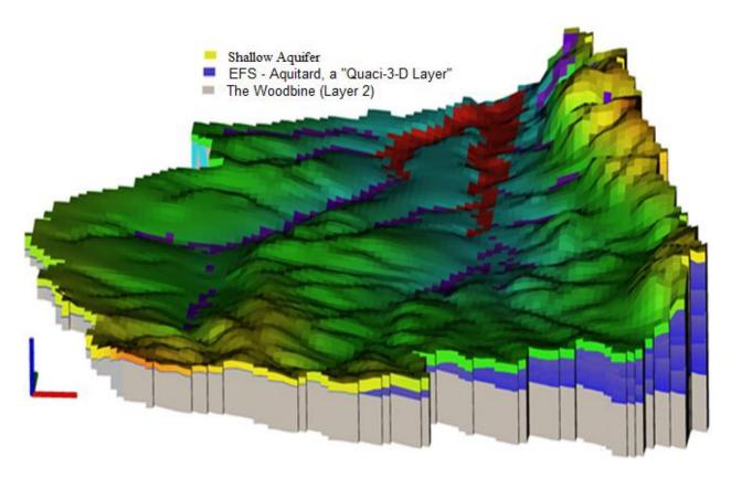
Figure 5-3 The vertical discretization of the JPL model; (Diagram is not to the Scale)
