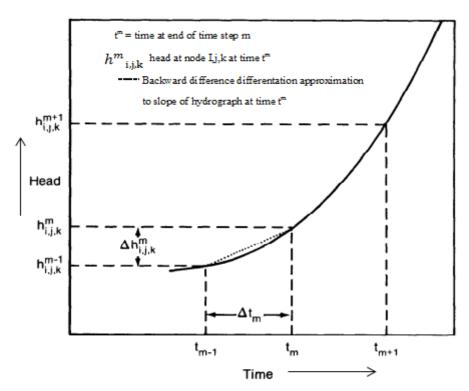
Figure B-3 Hydrograph for cell i,j,k used in backward-difference approach of finite-difference approximation (McDonald and Harbaugh,1988)
