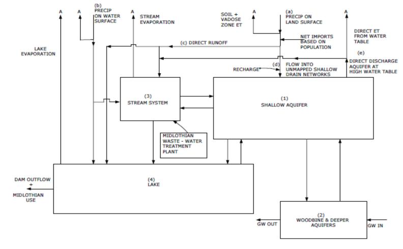
Figure 5-1 The schematic diagram illustrating the major components of the present-day hydrologic regime in the JPL catchment, and the role of the alluvial groundwater system within it
