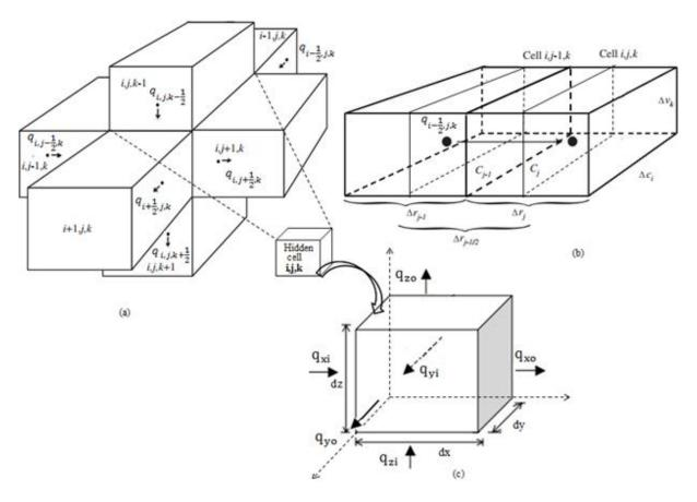
Figure B-1 Illustrating the conventions of cells used in finite-difference approximation of groundwater flow equation. Where, (a) three-dimensional representation of flow in MODFLOW simulation; the center of the cell i,j,k (hidden) is surrounded by six cells, (b) one dimensional groundwater flow into the cell i,j,k from an adjacent cell, and (c) the 3-D cube receiving flow from six adjacent cells
