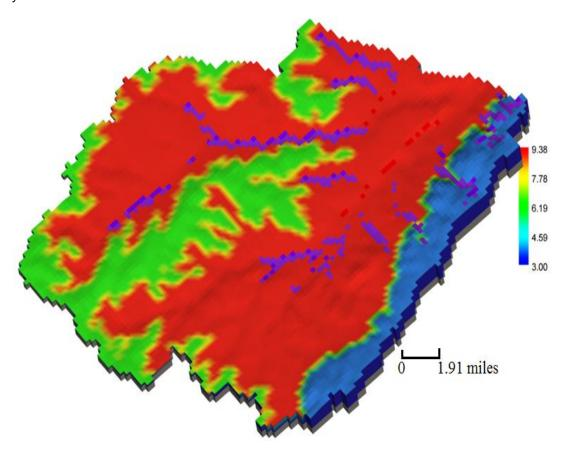
Figure 5-6 The horizontal hydraulic conductivity of shallow aquifer used in optimum simulations in pre-lake and post-lake conditions
