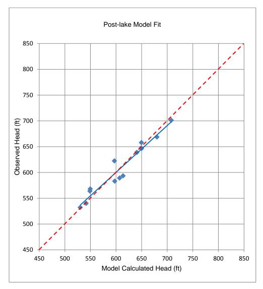
Figure 6-10 Post-lake model fit of JPL project MODFLOW simulation
