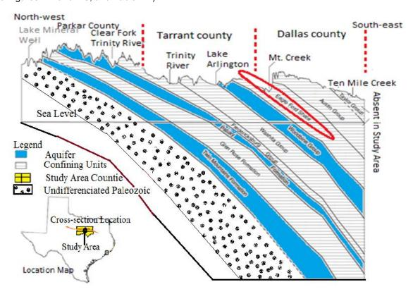
Figure 1-2 Generalized cross-section showing the consolidated rock units near the study area.
