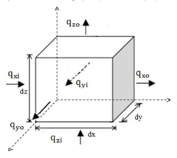
Figure A-1 Diagram showing three-dimensional groundwater flow in an infinitesimally small cube, a representative elementary volume (REV)
