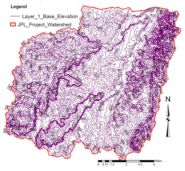
Figure 5-4 An approximate representation of the Layer 1 base elevation of the shallow groundwater aquifer of JPL groundwater simulation
