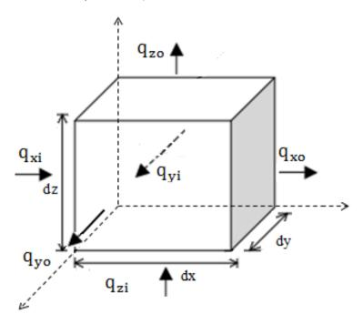
Figure 5-2 Diagram showing three-dimensional groundwater flow in an infinitesimally small cube, a representative elementary volume (REV)
