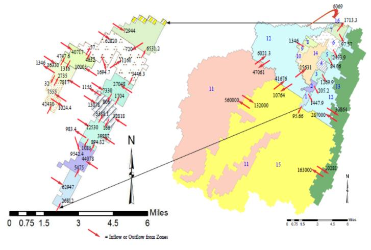
Figure 6-5 The distribution of horizontal flow between zones in the shallow groundwater aquifer under pre-lake conditions.
