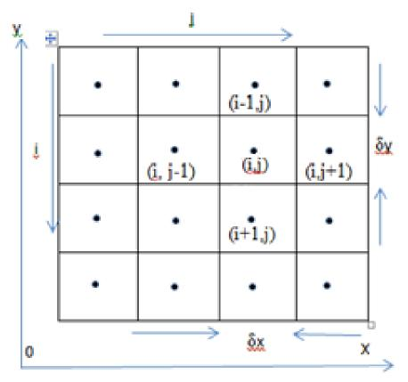
Figure B-4 Finite-difference grid representation for the flow in MODFLOW depicting the numbering convention (Wang and Anderson, 1982)
