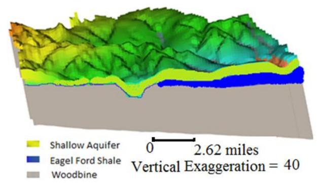
Figure 3-3 The model cross section along the column 55 that passes between the two arms of JPL
