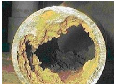
Figure 6 Example of Pitting Corrosion in pipes [22]
