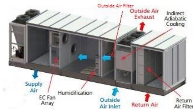
Figure 9 Indirect-Evaporative Air-Side Economizer Unit [14]
