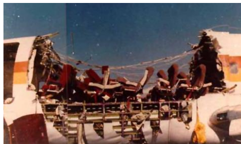
Figure 7 Example of Fatigue Corrosion [22]
