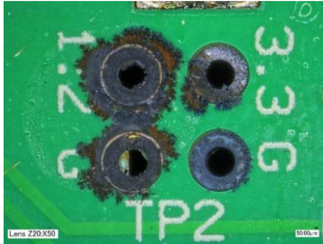
Figure 2 Short Due to the Mixture of Gaseous Contaminants
