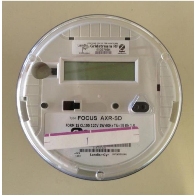
Figure 2-5 A Landis+Gyr FOCUS AXR-SD 120V Smart Meter, used in all tests throughout this study.
