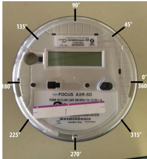
Figure 3-1 Angles marked on the Smart Meter for reference as to where measurements were taken in relation to position on the rotary table.
