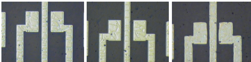
Figure 3.4 Optical microscope photos of thin films Pt/Cr/PI, Pt/Cu/Cr/PI and Pt/Au/Cr/PI (left to right).
