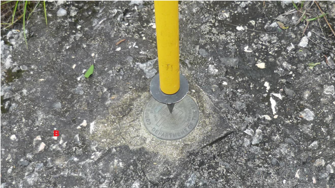
Figure A2. Photographs of site ARC1 acquired during May 2011 campaign. (A) Photoview facing west. (B) Geodetic monument at ARC1, the geodetic benchmark is inside a concrete slab cemented into local bedrock.
