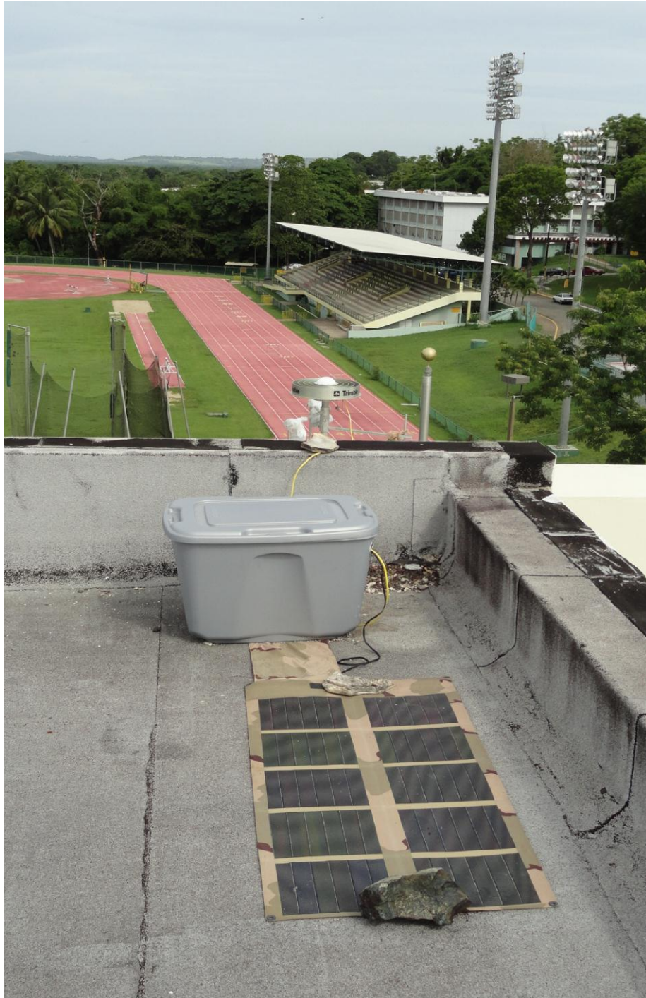
Figure 2.4 Geodetic setup with a solar backup on the campaign site LAJ1.
