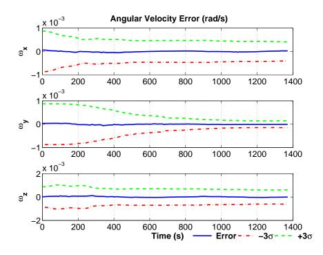
Figure 8.20. UKF Levenberg Marquardt Batch Estimation of Angular Velocity.
