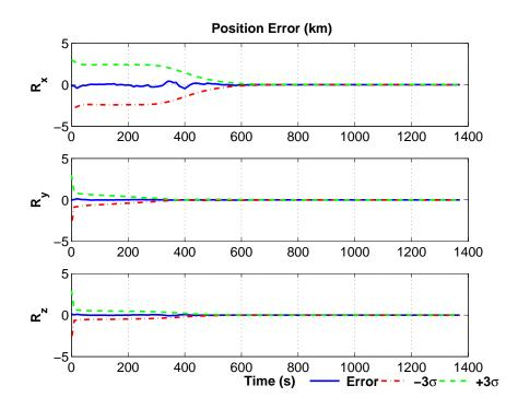
Figure 8.16. UKF Levenberg Marquardt Batch Estimation of Position.
