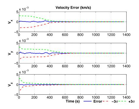
Figure 8.17. UKF Levenberg Marquardt Batch Estimation of Velocity.
