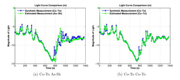
Figure 7.14. Inverse Problem Acquired vs. Estimated Light Curve Measurement.
