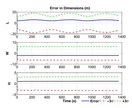
Figure 9.12. BPF Joint Estimation of Shape/Size Parameters.
