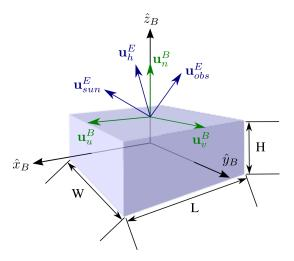
Figure 4.2. Resident Space Object Model with Light Curve Model Vectors.
