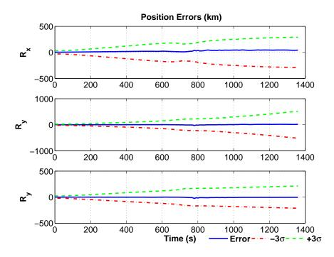
Figure 9.7. BPF Joint Estimation of Position.
