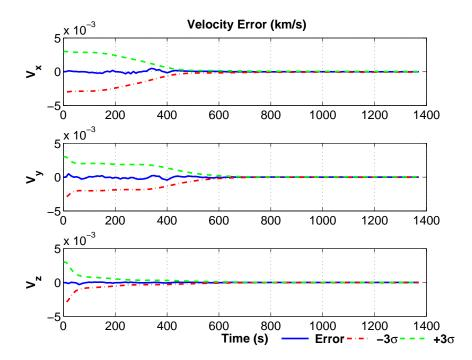
Figure 8.10. UKF Joint Estimation of Velocity.
