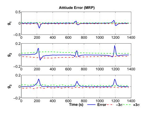
Figure 8.11. UKF Joint Estimation of Attitude (MRPs).
