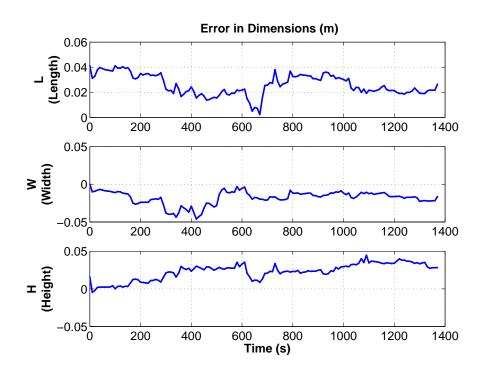
Figure 8.15. UKF Joint Estimation of Shape/Size Parameter (no  $3\sigma$  bounds).
