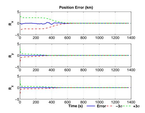
Figure 8.23. UKF Gauss Newton Batch Estimation of Position.
