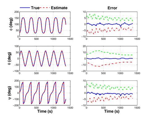
Figure 8.12. UKF Joint Estimation of Attitude (Euler Angles).
