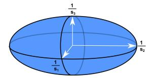
Figure 6.1. Depiction of Observability Degree for a Three Dimensional Vector.
