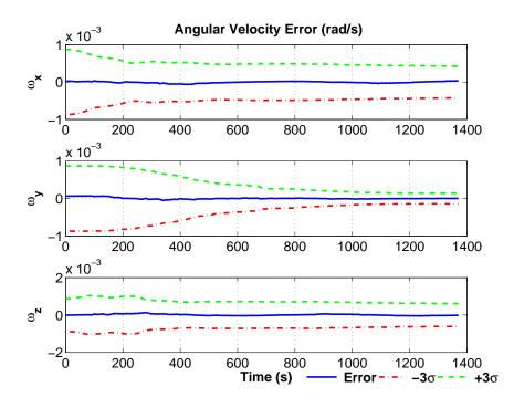
Figure 8.13. UKF Joint Estimation of Angular Velocity.
