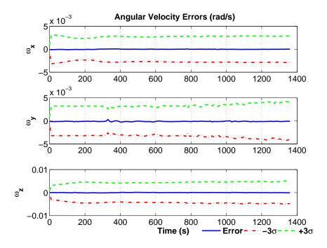
Figure 9.11. BPF Joint Estimation of Angular Velocity.
