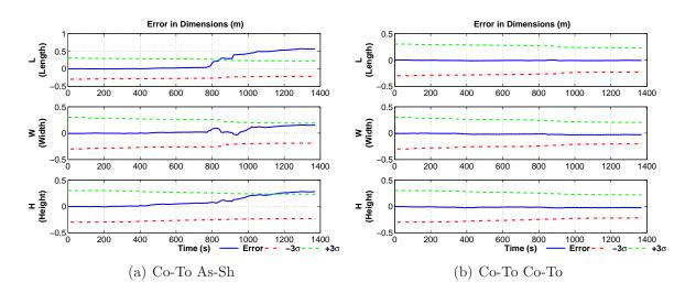
Figure 7.12. Inverse Problem Estimation of Shape/Size Parameters.
