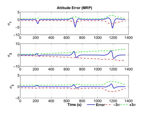
Figure 9.9. BPF Joint Estimation of Attitude (MPRs).
