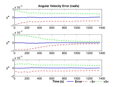
Figure 8.27. UKF Gauss Newton Batch Estimation of Angular Velocity.
