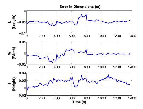
Figure 8.21. UKF Levenberg Marquardt Batch Estimation of Shape/Size Parameters.
