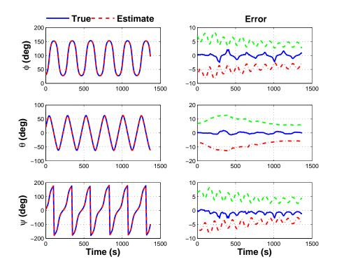
Figure 8.26. UKF Gauss Newton Batch Estimation of Attitude (Euler Angles).
