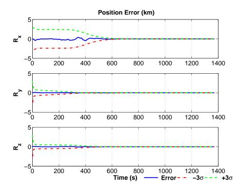
Figure 8.9. UKF Joint Estimation of Position.
