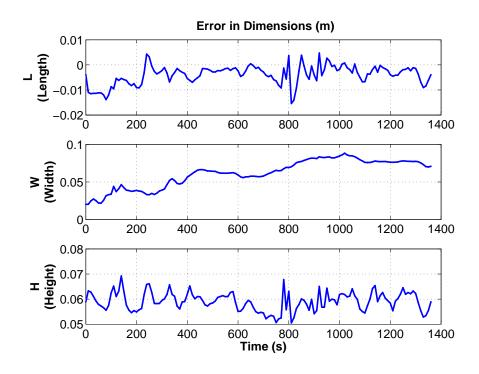
Figure 9.13. BPF Joint Estimation of Shape/Size Parameter (no  $3\sigma$  bounds).
