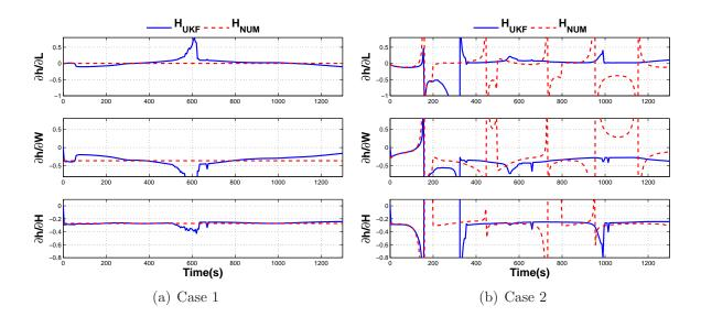
Figure A.8. Ward-Dür Model Shape/Size Parameters Sensitivity.
