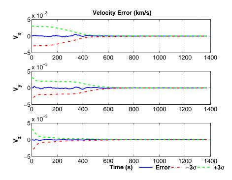
Figure 8.24. UKF Gauss Newton Batch Estimation of Velocity.
