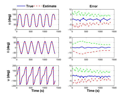
Figure 8.19. UKF Levenberg Marquardt Batch Estimation of Attitude (Euler Angles).
