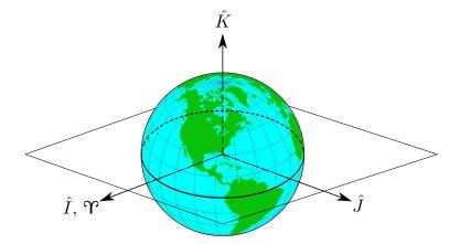
Figure 2.1. Earth Centered Inertial Frame.
