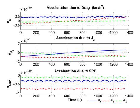
Figure 9.5. BPF Joint Estimation Perturbation Accelerations.
