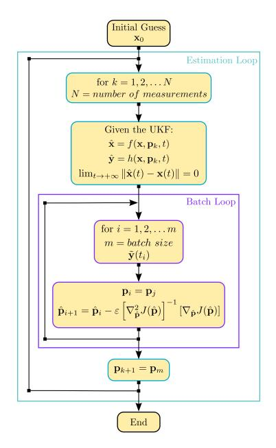
Figure 8.1. UKF-Batch Estimation Algorithm.
