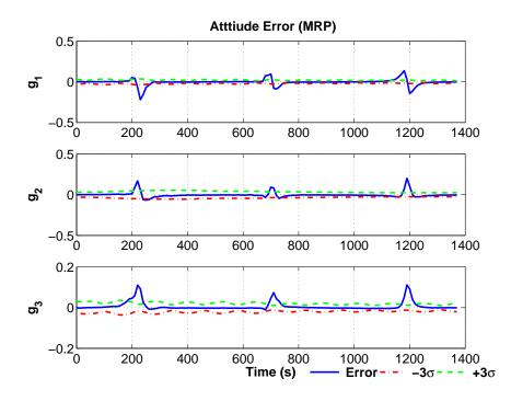
Figure 8.18. UKF Levenberg Marquardt Batch Estimation of Attitude (MRPs).
