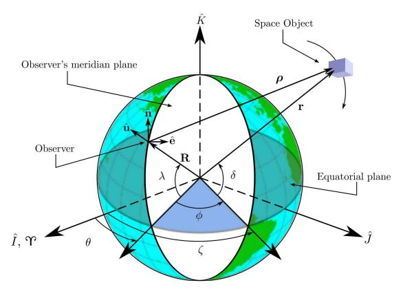
Figure 4.1. Geometry of Earth, Observer, and Object.
