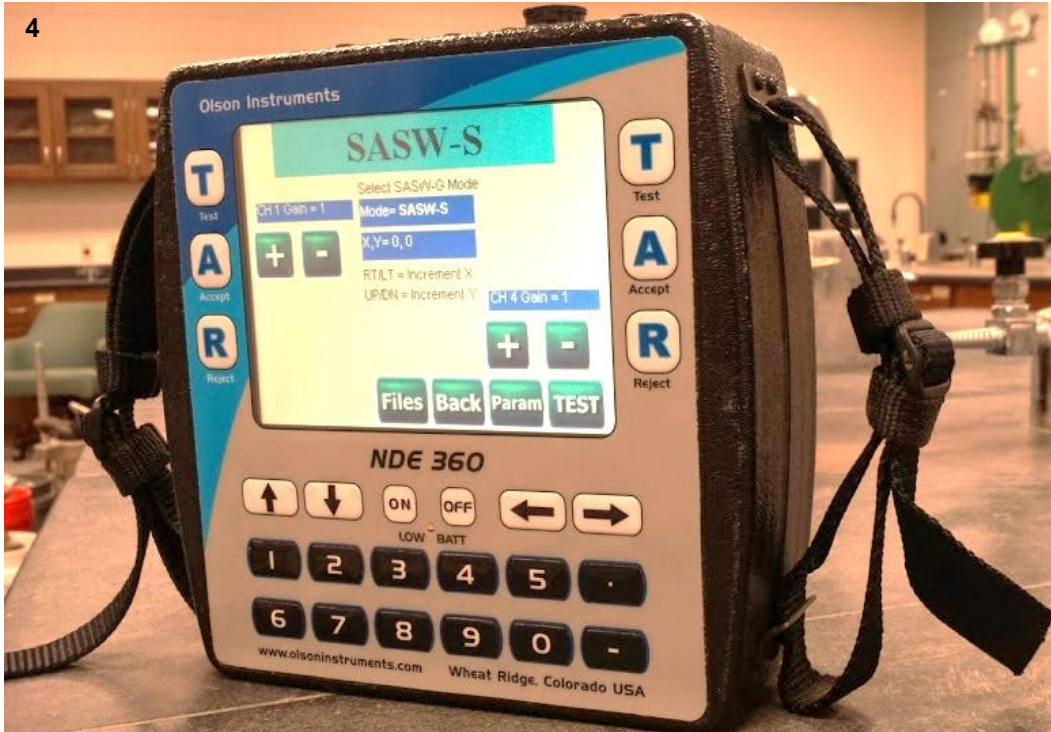
Figure 3- 12 Data Logger (NDE 360)
