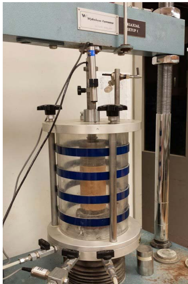
Figure 3- 3 Test set-up for UCS test
