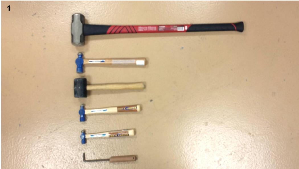
Figure 3- 9 Various Hammers used to provide Impact
