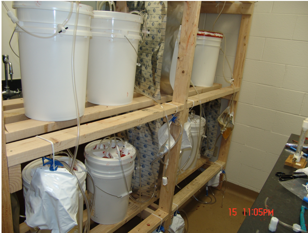
Figure 3.2 Two sets of bioreactor cells with and without soil representing the four phases of decomposition (Hossain et al, 2007).
