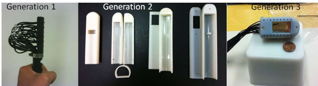
Figure 5-7 pictures showing various generations of the optical Clip-on probes developed
