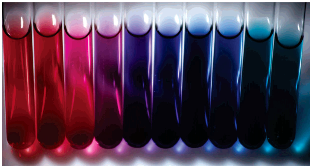
Figure 2.6 (a) UV-VIS absorption spectra of nine hollow gold nanoparticle samples with varying diameters and wall thicknesses. (b) Image showing the color range of hollow gold nanoparticle solutions. The vial on the far left contains solid gold nanoparticles, the rest are hollow gold nanoparticles with varying diameters and wall thicknesses.
