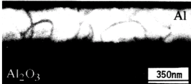
Figure 2-14 Cross sectional TEM image of a 350nm thick epitaxial Al film deposited on a single crystal (0001) alpha- \text{Al}_2\text{O}_3 substrate during heating.
