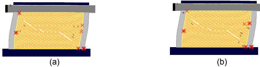
Figure 4.34 Cracking patterns at 1.0% drift for second set specimens with different transverse steel spacing. (a) P2Dp5 and (b) P2Dp25.
