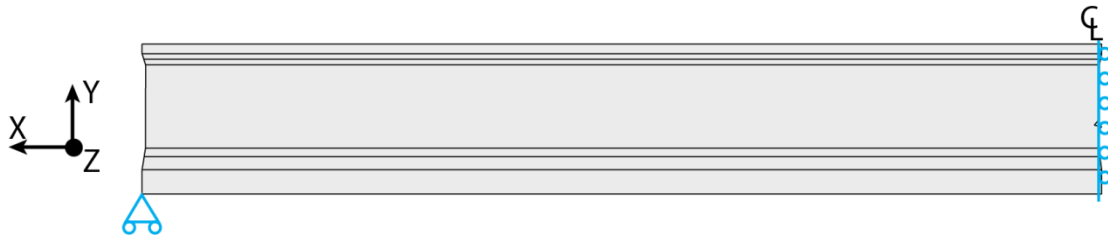
Figure 5.8: Boundary conditions of finite element model.
