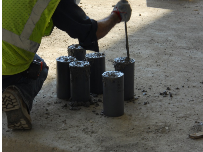
Figure 2.25: Collection of concrete cylinders.
