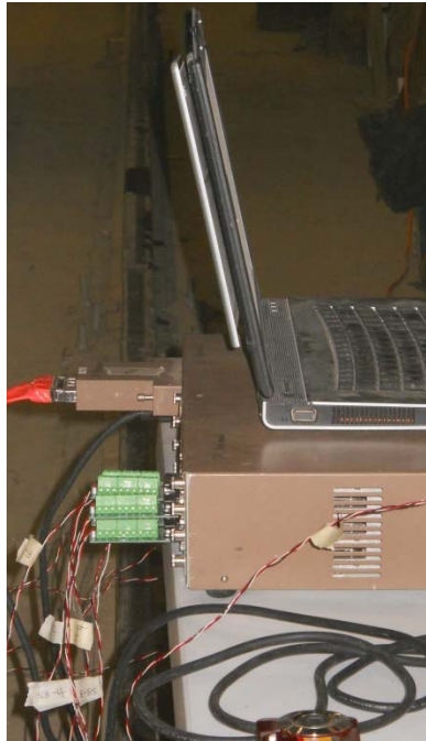
Figure 3.5: Strain reader connected to the computer.
