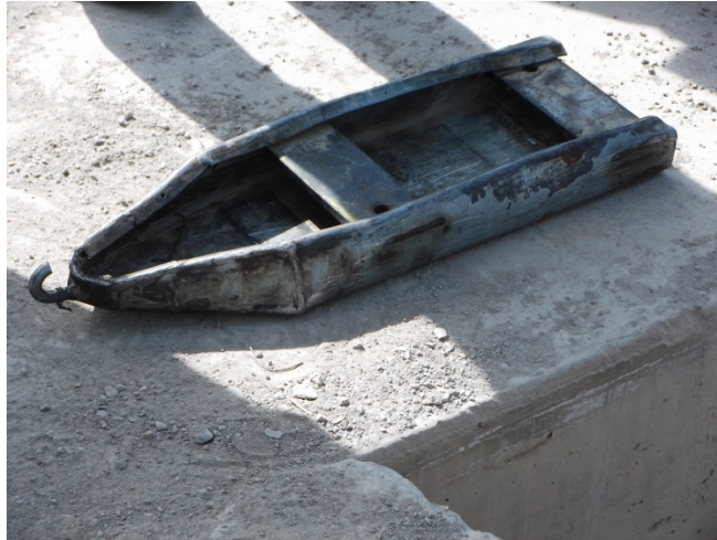
Figure 2.16: Device used to place the strands along the girder.
