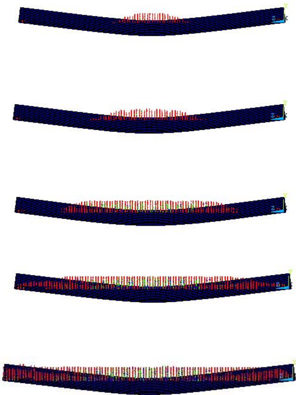
Figure 4-22 Progression of Cracks with Load Increment for Prestressed Concrete I-Girder Strengthened for Shear
