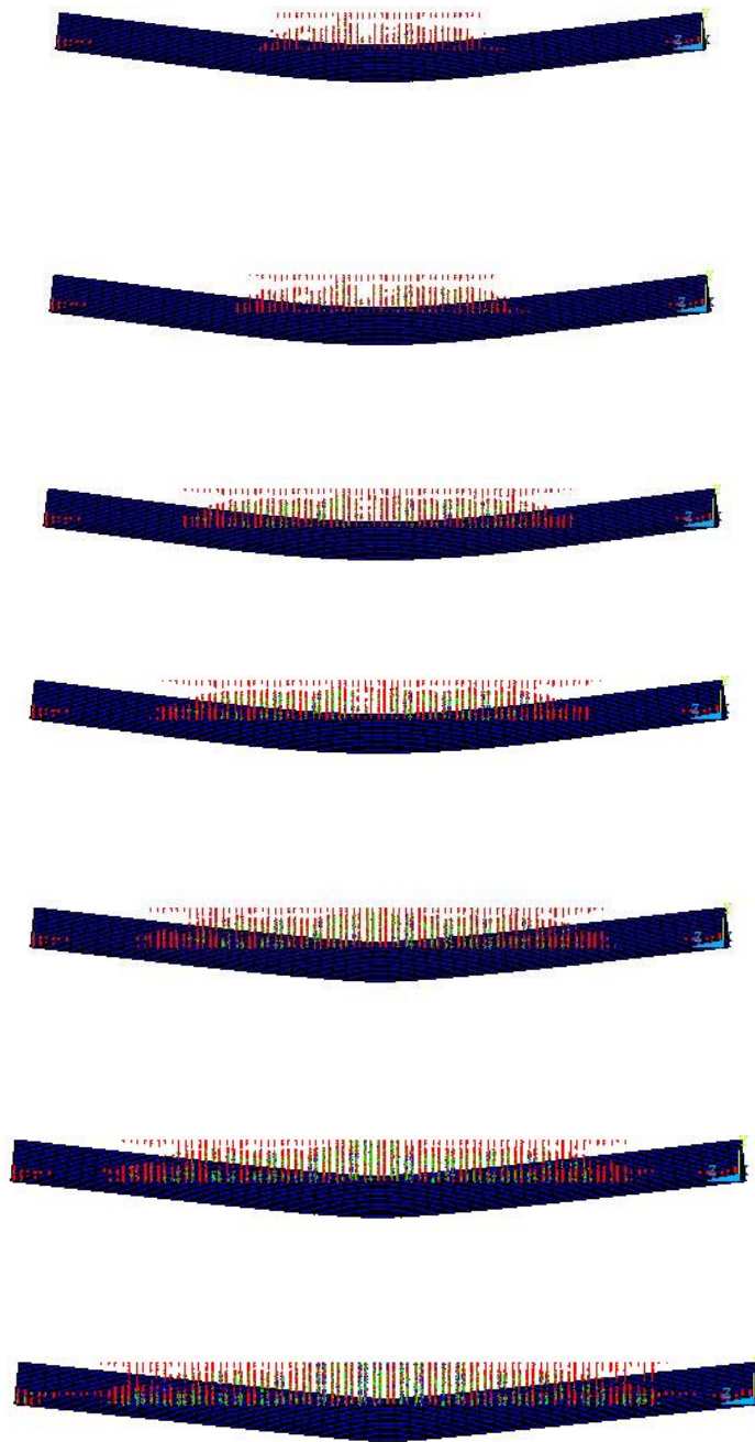
Figure 4-6 Progression of Cracks with Load Increment for Prestressed Concrete I-Girder
