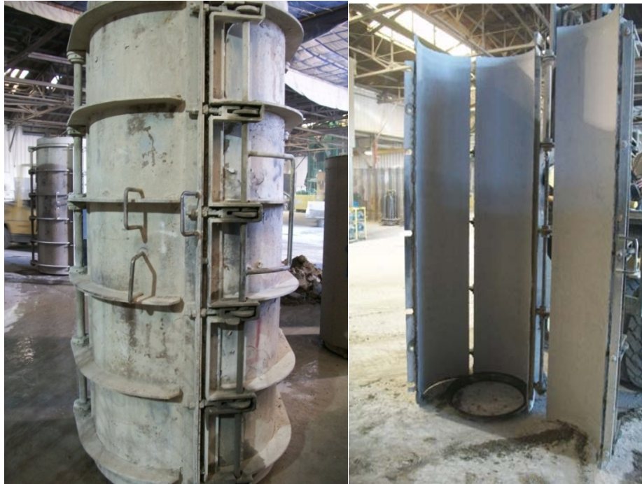
Figure 1-8 Photograph of Three-piece Jacket (metal pipe form) at Hanson Facility
