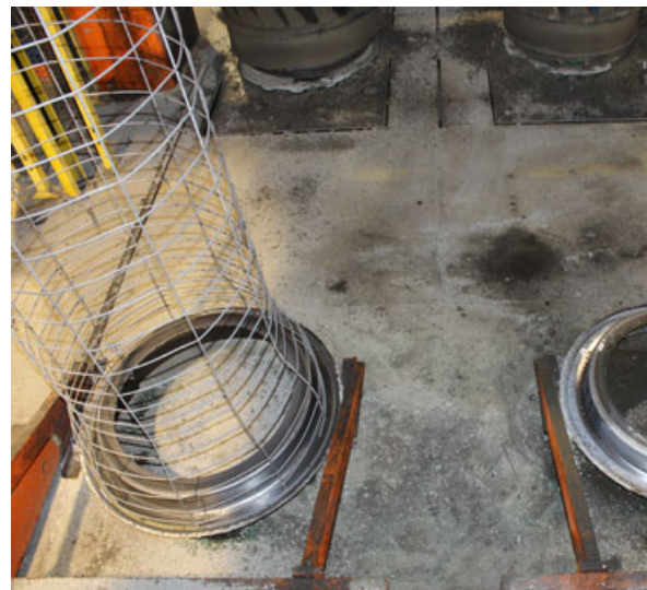
Figure 1-5 Photograph of steel cage after production (Courtesy of: http://www.langleyconcretegroup.com/uploads/images/tour/Mastematic%20-%20Automated%20pipe%20production/8---The-pallet-automation-moves-the-pallets-forward-where-the-reinforcing-cage-is-placed-on-the-pallet,-where-needed..jpg )
