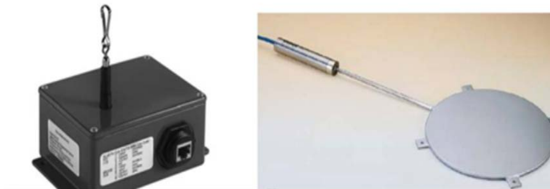
Figure 2-22 Sensors for long-term monitoring; (a) cable displacement sensor (CDS), (b) Pressure transducer (semi-conductor type)
