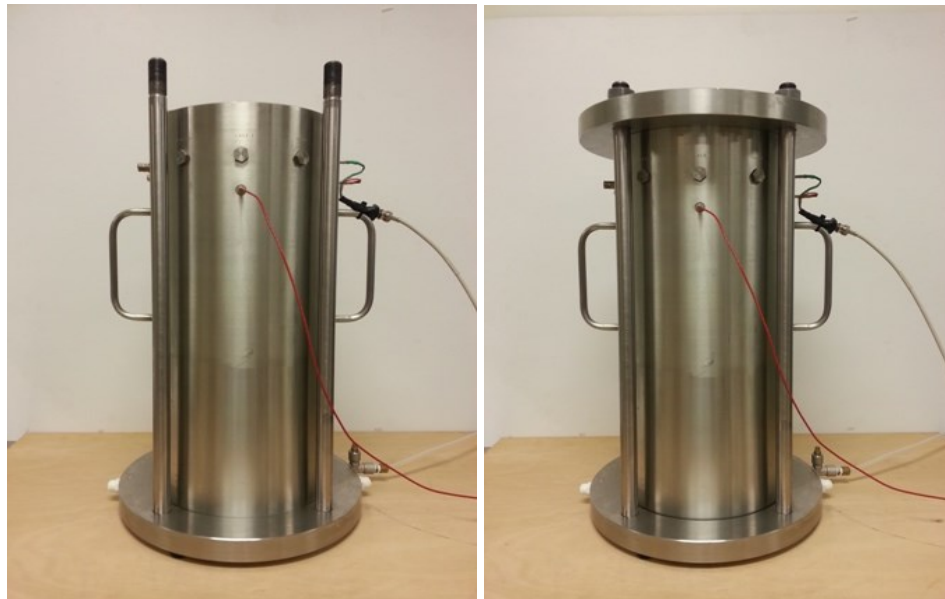
Figure 3-5 fully assembled confining chamber
