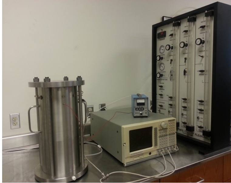
Figure 3-6 fully assembled resonant column test setup
