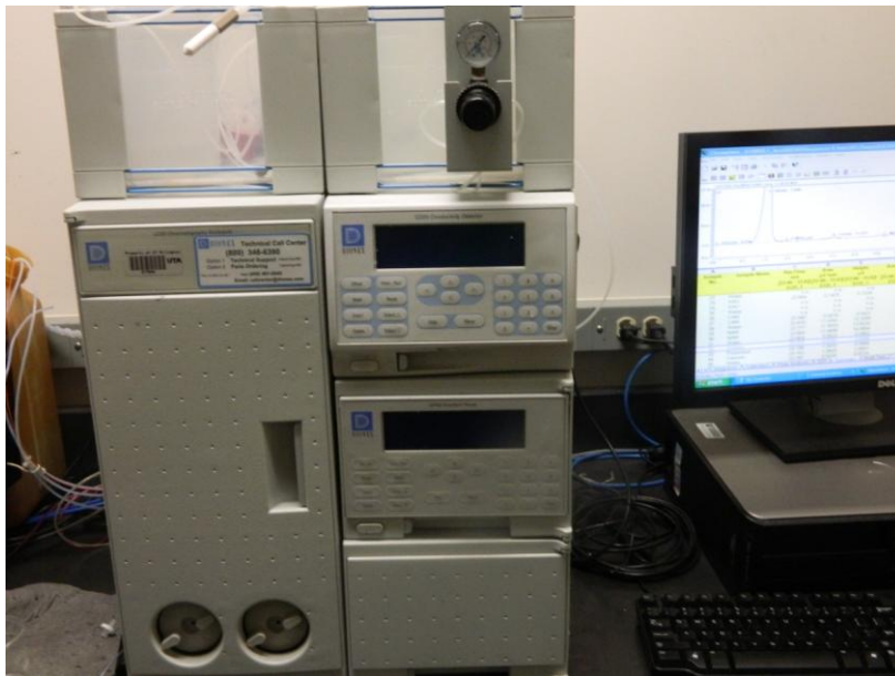
Figure 3.5 Ion chromatography (IC) test equipment
