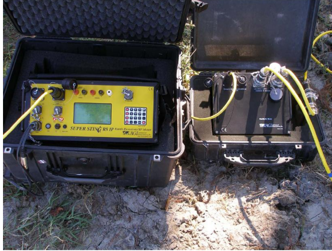
Figure 7.4 Super Sting R8/IP multichannel system and switch box
