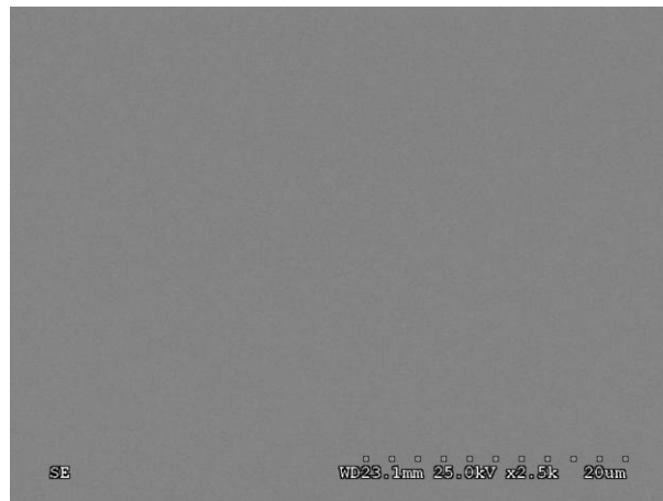
Figure 4-25 SEM of TaN film deposited at a substrate bias of -200 V, 5% N 2 and deposition temperature 350°C
