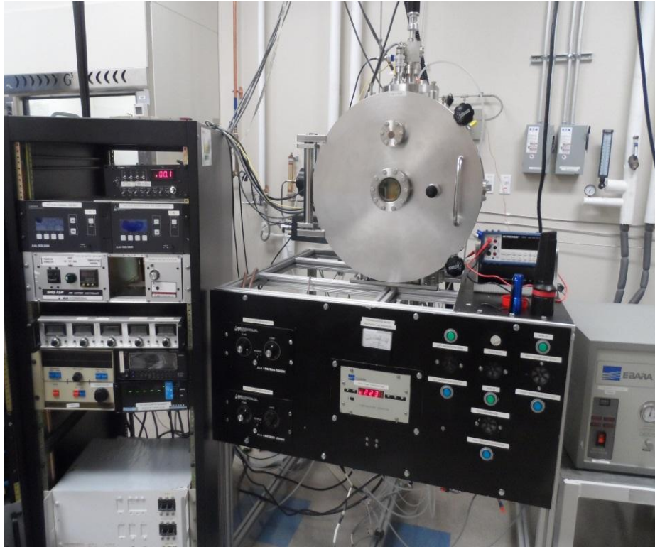
Figure 3-1 PVD reactive magnetron sputtering system in Surface and Nano Engineering Laboratory
