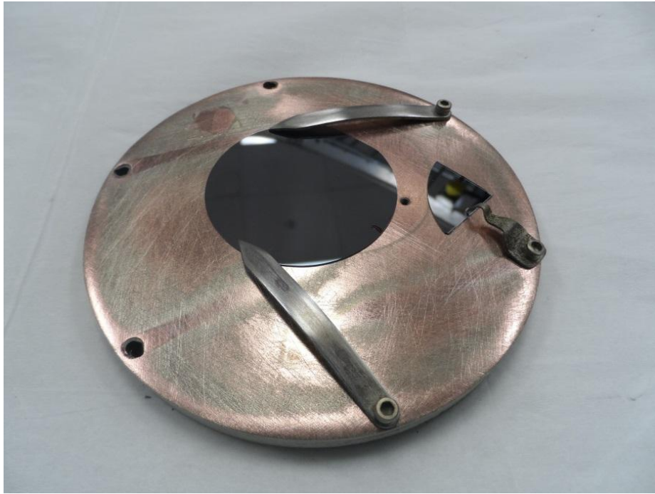
Figure 3-2 Silicon wafer loaded on the substrate holder
