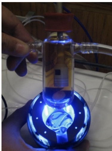
Figure 2.5 Photoreactor as used in photolysis experiments for photoreduction of carbon dioxide.
