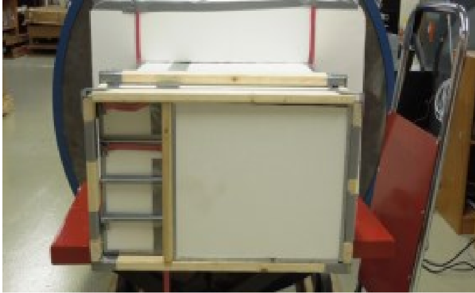
Figure 6.1: Fan wall built to mount the 80mm fan wall array
