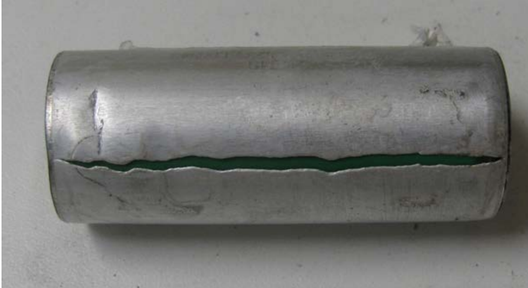
Figure 23 failed 26650 cell after a 75A (50C) charge.
