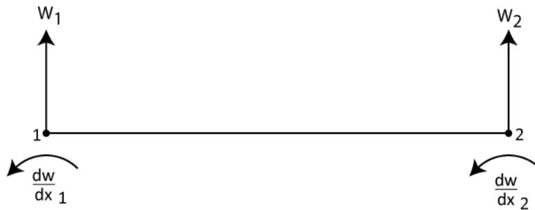
Figure 3.2 Two-Node Timoshenko Beam Element with Four-Degrees of Freedom
