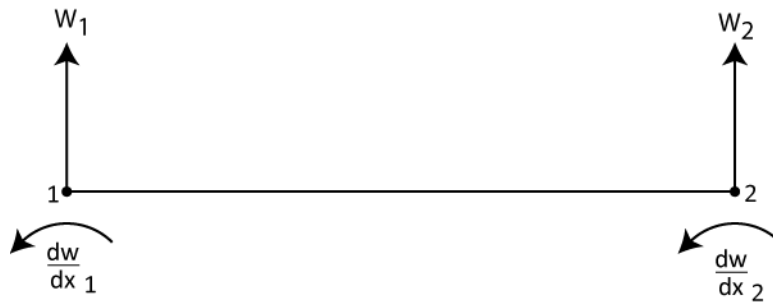
Figure 2.4 Two-Node Timoshenko Beam Element
