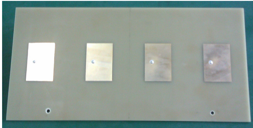
Figure 4-7 Photo of the fabricated 4-element antenna array.
