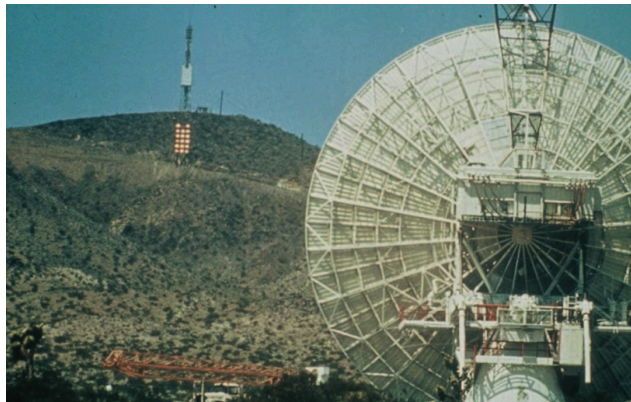
Figure 2-11 First ground-to-ground microwave beam wireless power transmission experiment in 1975 at the Venus Site of JPL Goldstone Facility [74].
