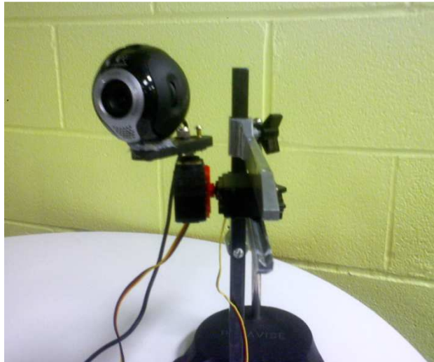
Figure 4.1 Robot with two degrees of freedom (Pan and tilt)
