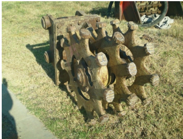
Figure 2 - 32 Sheep foot roller compactor
