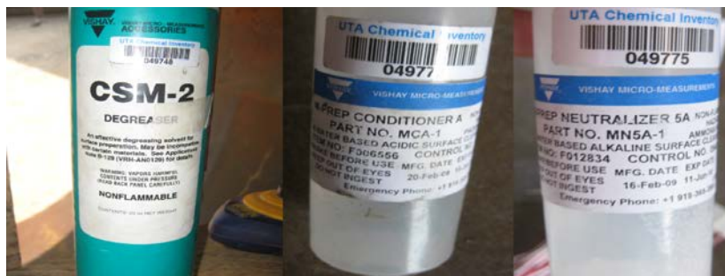
Figure 2 - 9 Surface chemical cleaning preparation
