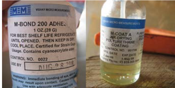
Figure 2 - 10 Adhesive and protective coating
