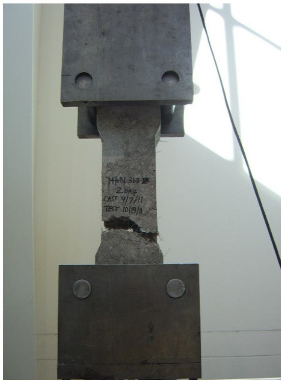
Figure E- 12 Crack formation of HAN36-8-B-88(2)-T1-DT
