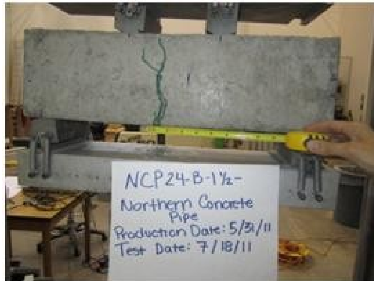
Figure D- 42 Crack pattern for NCP24-8-B-0.5-T2-BM
