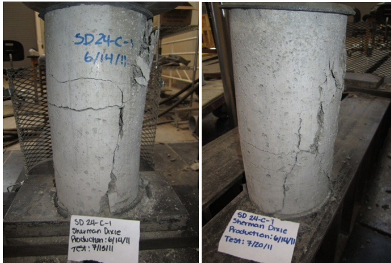
Figure C- 3 Typical failure mode of SHD cylinder with 0.33%
