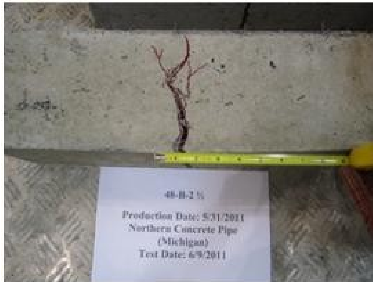
Figure D- 62 Crack pattern for NCP48-8-B-0.83-T1-BM
