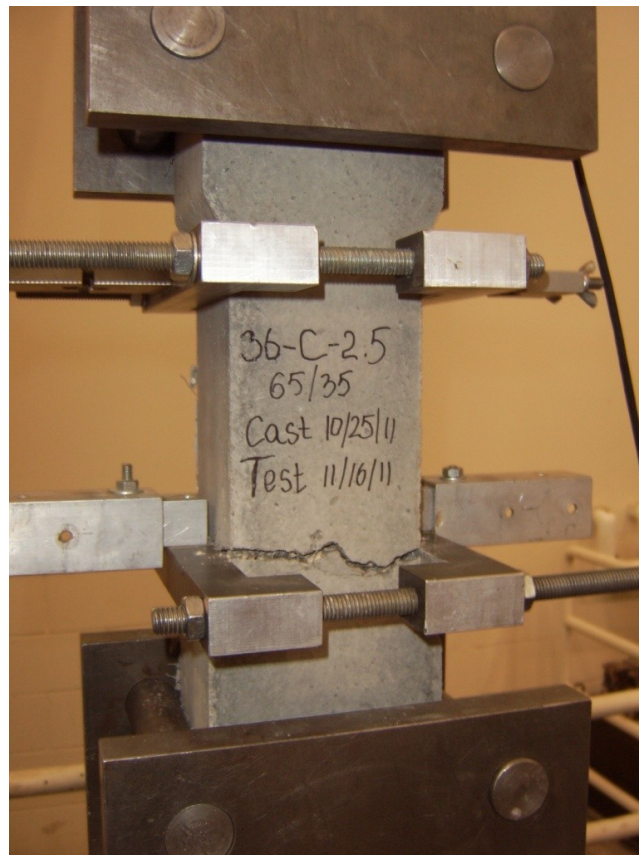
Figure E- 14 Crack formation of HAN36-8-C-110(2 ½)-T1-DT
