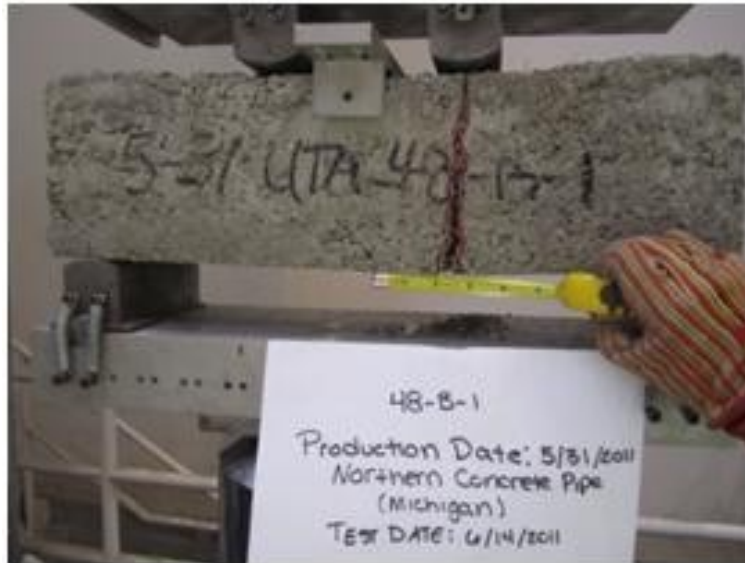
Figure D- 24 Crack pattern for NCP48-8-B-0.33-T1-BM
