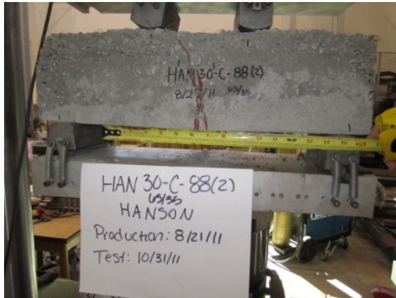
Figure D- 48 Crack pattern of HAN30-8-C-0.67-T1-BM
