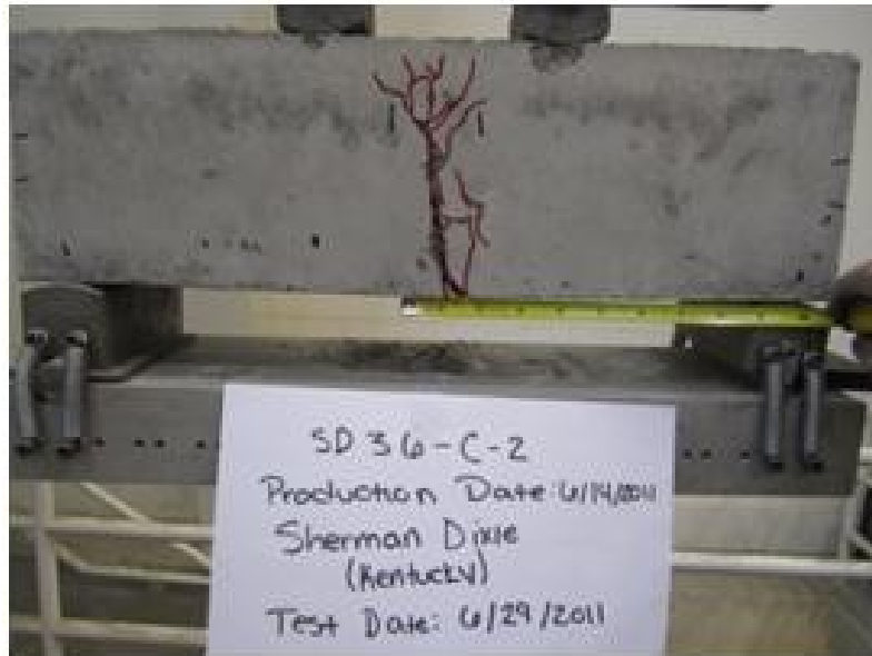
Figure D- 54 Crack pattern for SHD36-8-C-0.67-T1-BM
