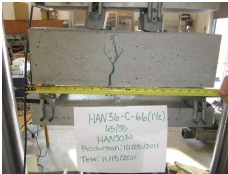
Figure D- 32 Crack pattern of HAN36-8-C-0.5-T2-BM
