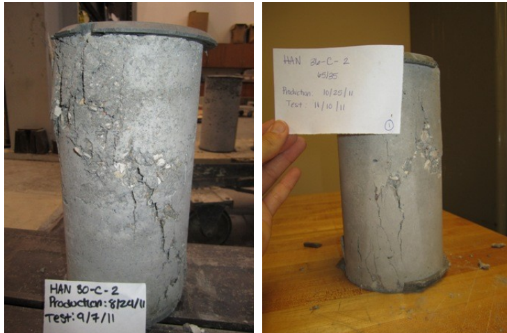
Figure C- 15 Typical failure mode of HAN cylinder with 0.67%
