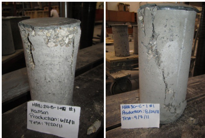
Figure C- 13 Typical failure mode of HAN cylinder with 0.33%
