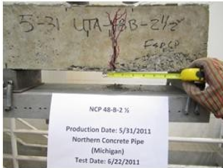
Figure D- 64 Crack pattern for NCP48-8-B-0.83-T2-BM
