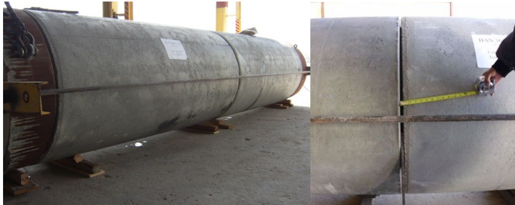
Figure 2-13 Hydrostatic test setup at deflected 1/2" position
