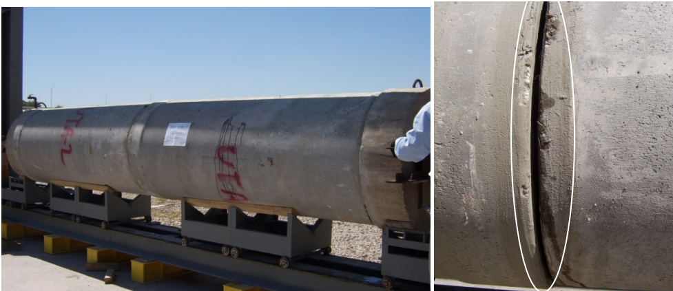
Figure B- 56 Specimen 3 for HAN-30-C-0.5 SFRCP dripping from the body and joints
