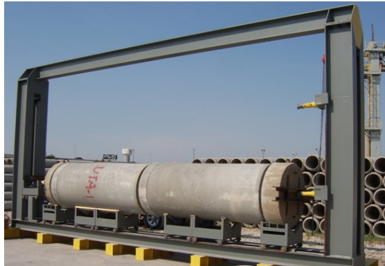
Figure 2-25 Hydrostatic test setup in Grand Prairie, TX
