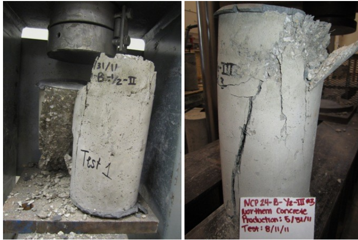
Figure C- 7 Typical failure mode of NCP cylinder with 0.17
