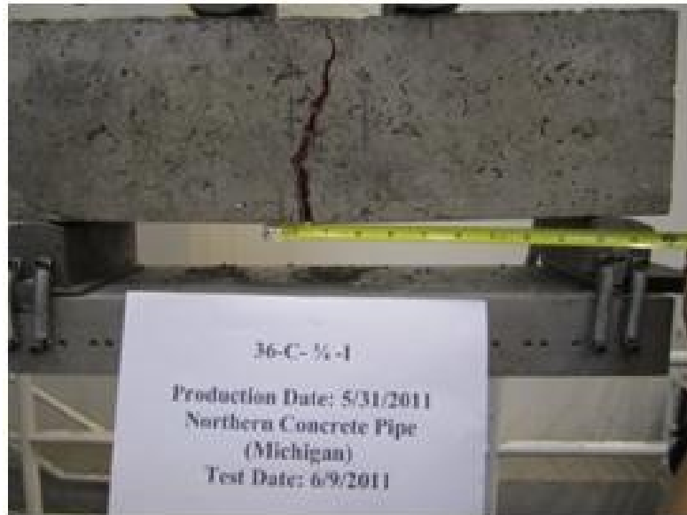
Figure D- 10 Crack pattern for NCP-36-8-C-0.25-T1
