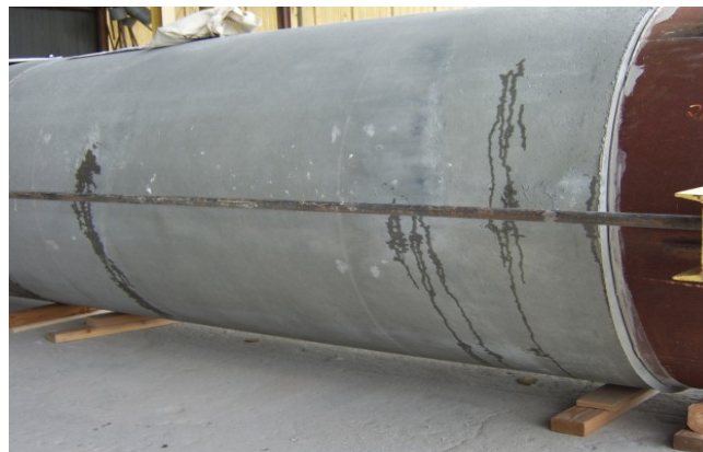
Figure B- 57 Specimen 4 for HAN-36-C-0.83 SFRCP seepage developed at seven locations
