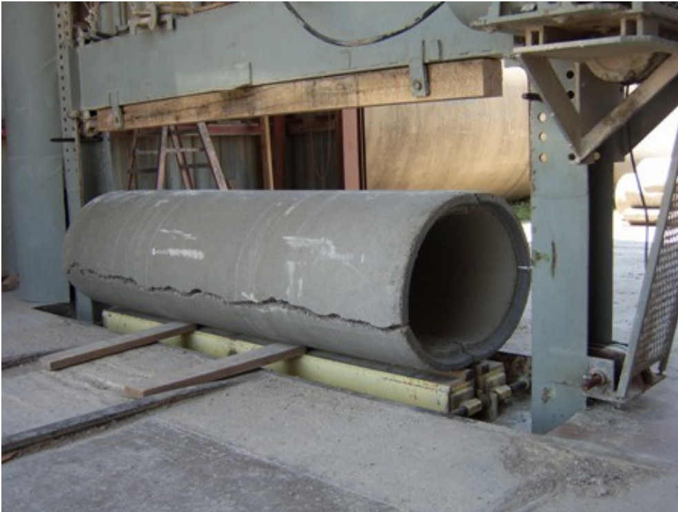
Figure B- 51 SFRCP 24 in. (600 mm) with 0.33% fiber fraction at large deformation
