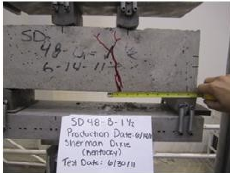
Figure D- 38 Crack pattern for SHD48-8-B-0.5-T1-BM
