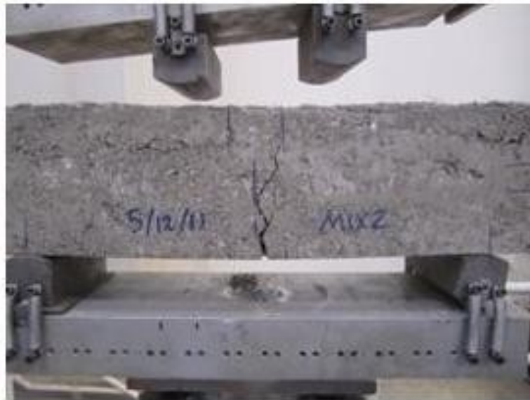
Figure D- 12 Crack pattern of HAN-24-8-B-0.33-T1
