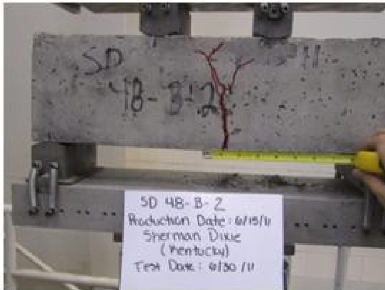
Figure D- 56 Crack pattern for SHD48-8-B-0.67-T1-BM
