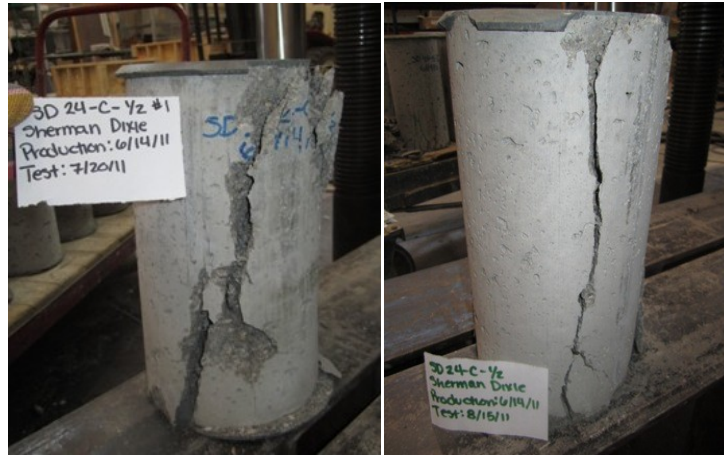
Figure C- 1 Typical failure mode of SHD cylinder with 0.17%
