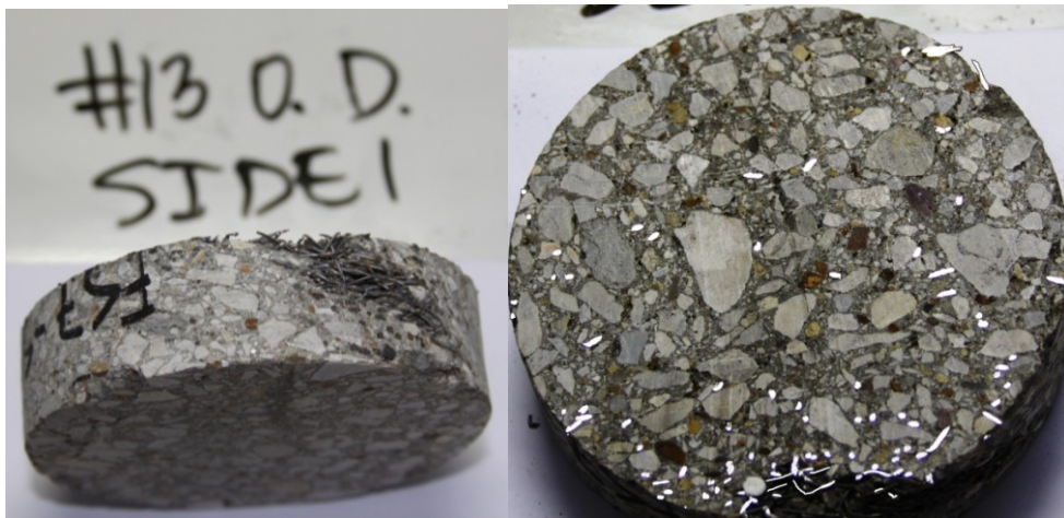
Figure 6-7 Fiber clustering in 24-B-0.33 (FS7) specimen
