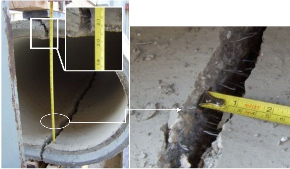
Figure B- 50 SFRCP 24 in. (600 mm) with 0.33% fiber fraction at 2.5 in deformation
