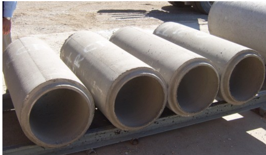
Figure 2-9 First SFRCP with 15 in. diameter lined up for testing
