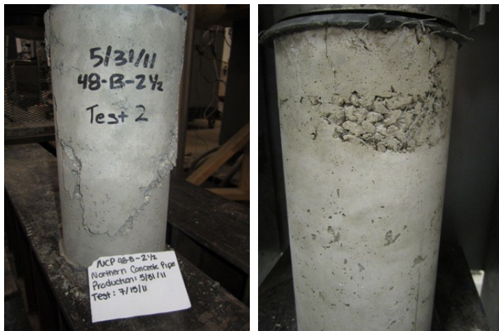
Figure C- 11 Typical failure mode of NCP cylinder with 0.83
