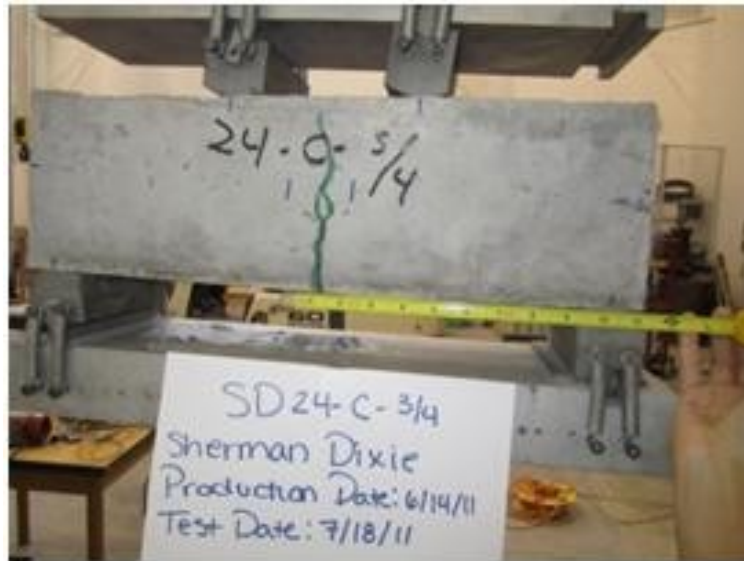
Figure D- 8 Crack pattern of SHD-24-C-0.25-T1
