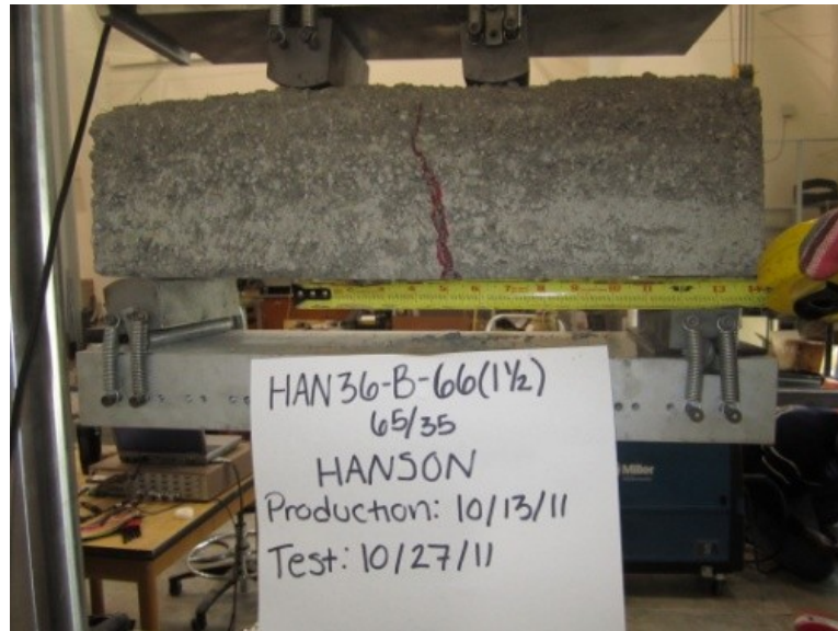
Figure D- 26 Crack pattern of HAN36-6-B-0.5-T1-BM
