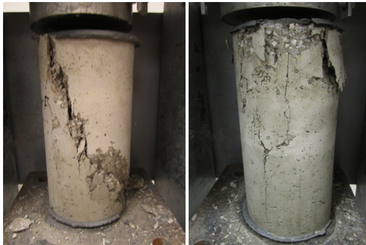
Figure C- 8 Typical failure mode of NCP cylinder with 0.25
