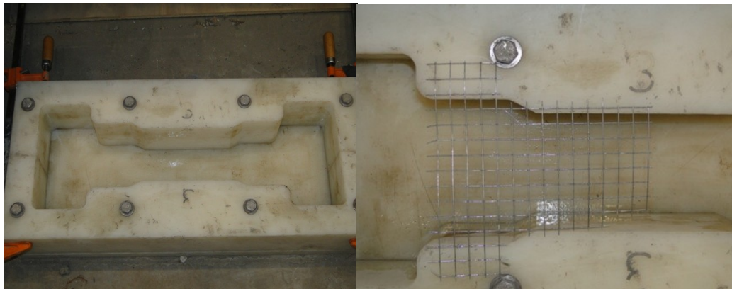
Figure 3-3 Direct tension test specimen mold on left and steel mesh reinforcing
