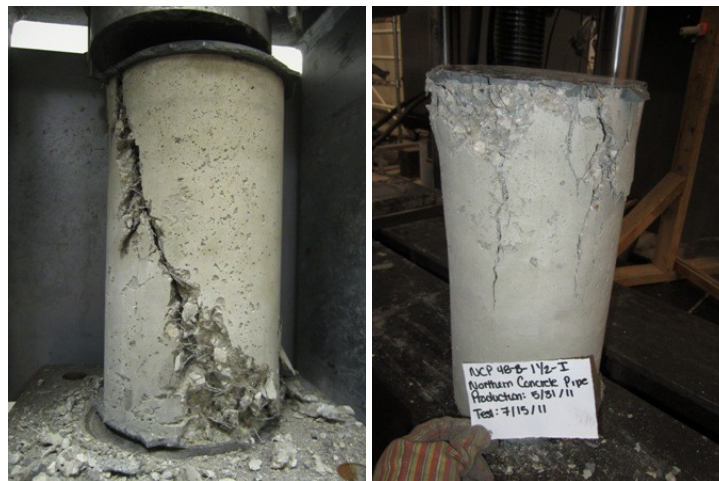
Figure C- 10 Typical failure mode of NCP cylinder with 0.5
