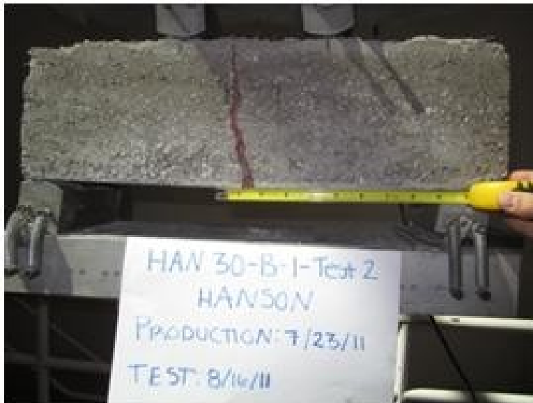
Figure D- 16 Crack pattern of HAN-30-B-0.33-T2
