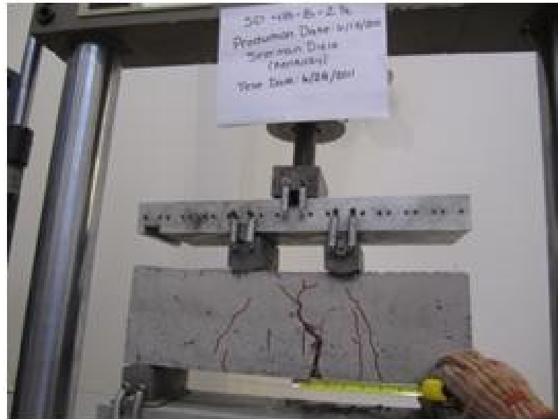
Figure D- 60 Crack pattern for SHD48-8-B-0.83-T1-BM
