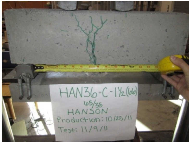
Figure D- 30 Crack pattern of HAN36-8-C-0.5-T1-BM
