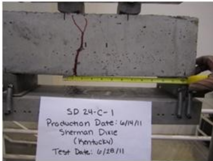
Figure D- 18 Crack pattern of SHD-24-C-0.33-T1
