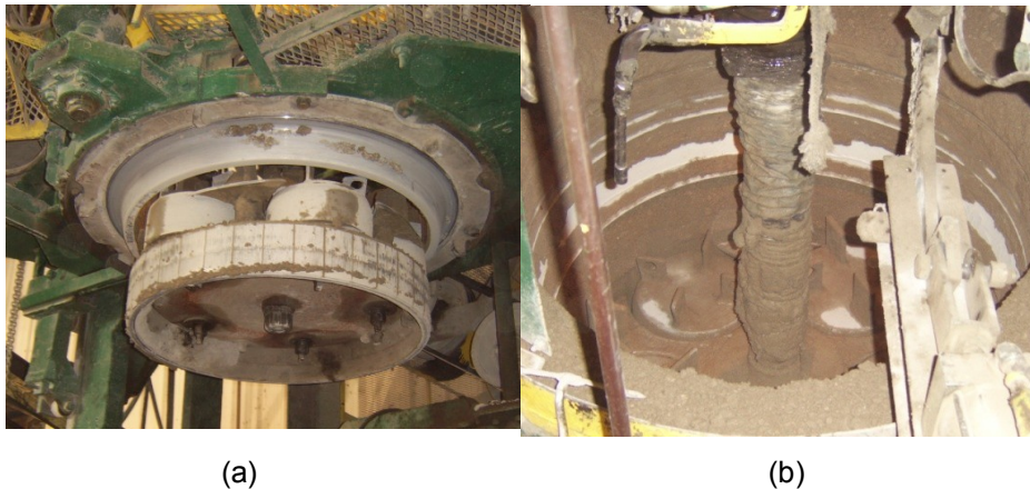
Figure 2-3 a) Roller head, (b) formation of inner surface of the pipe
