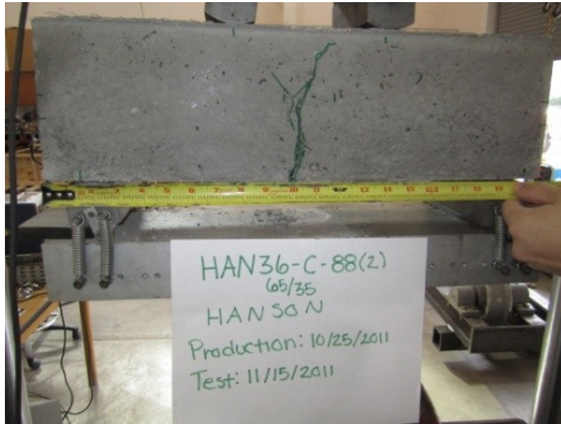
Figure D- 50 Crack pattern of HAN36-8-C-0.67-T1-BM
