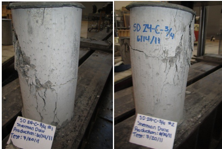
Figure C- 2 Typical failure mode of SHD cylinder with 0.25%
