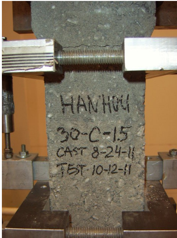
Figure E- 8 Crack formation of HAN30-8-C-66(1 1/2)-T1-DT
