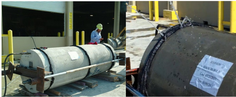
Figure 2-24 Hydrostatic testing on tongue and groove pipes using RAM-NEK
