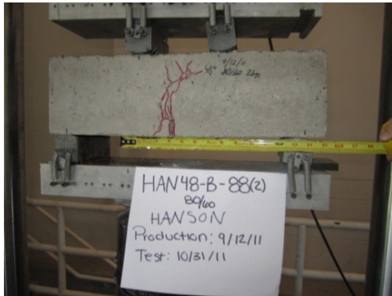
Figure D- 46 Crack pattern of HAN48-8-B-0.67-T1-BM
