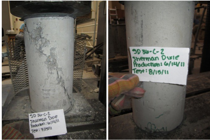
Figure C- 5 Typical failure mode of SHD cylinder with 0.67%
