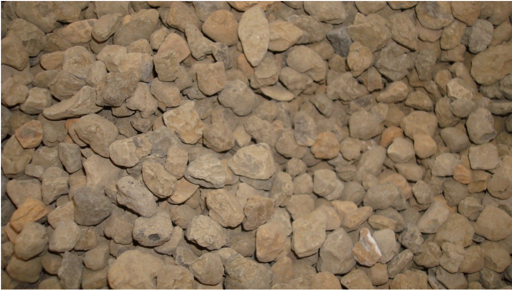
Figure 3-1 3/4" Expanded Shale Streetman Aggregate from ESCSI
