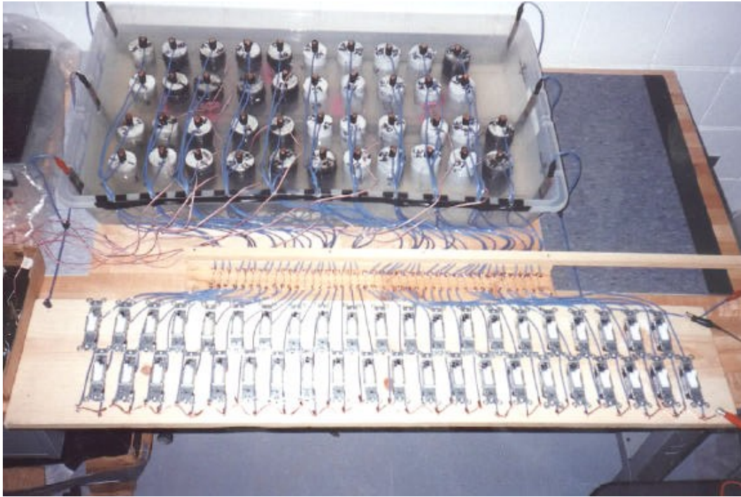
Figure 2-1 Accelerated Corrosion Experiment (Spainhour 2002)
