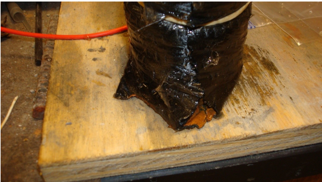
Figure 4-5 FRP rupture in Sample 21
