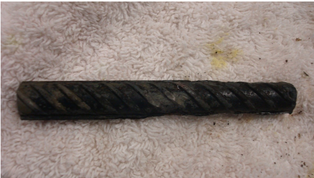
Figure 3-18 Rebar after corrosion removal
