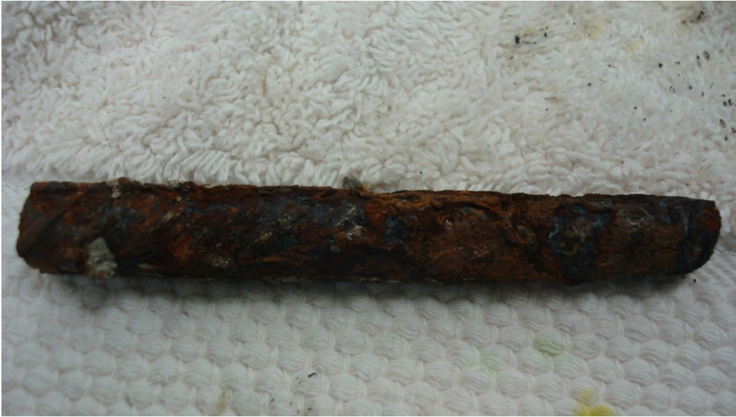
Figure 3-17 Rebar before corrosion removal
