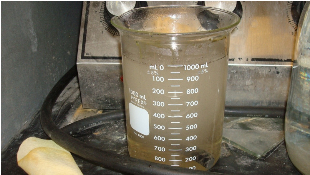
Figure 3-16 Rebar submerged in acid
