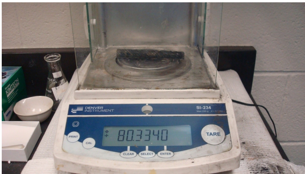
Figure 3-19 Weighing the cleaned rebar
