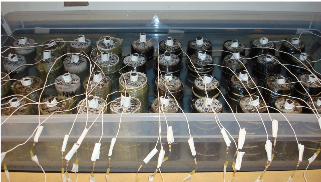
Figure 3-11 Samples completely wired and partially submerged in salt solution
