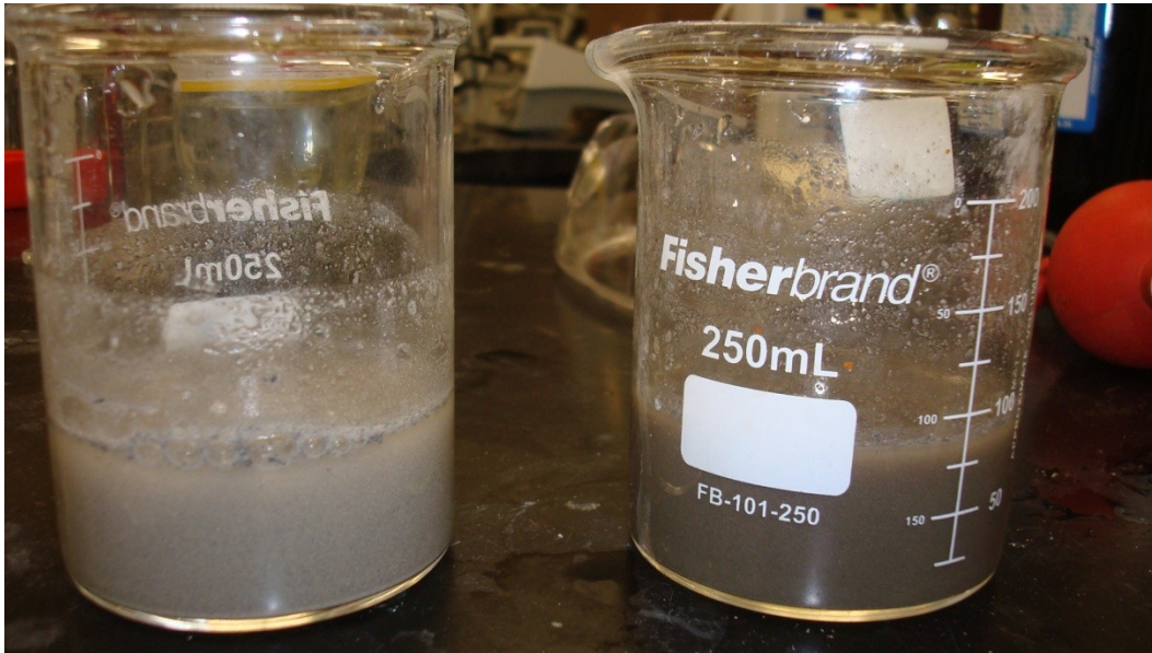
Figure 3-13 Concrete sample dispersed with water (NW on left, LW on right)
