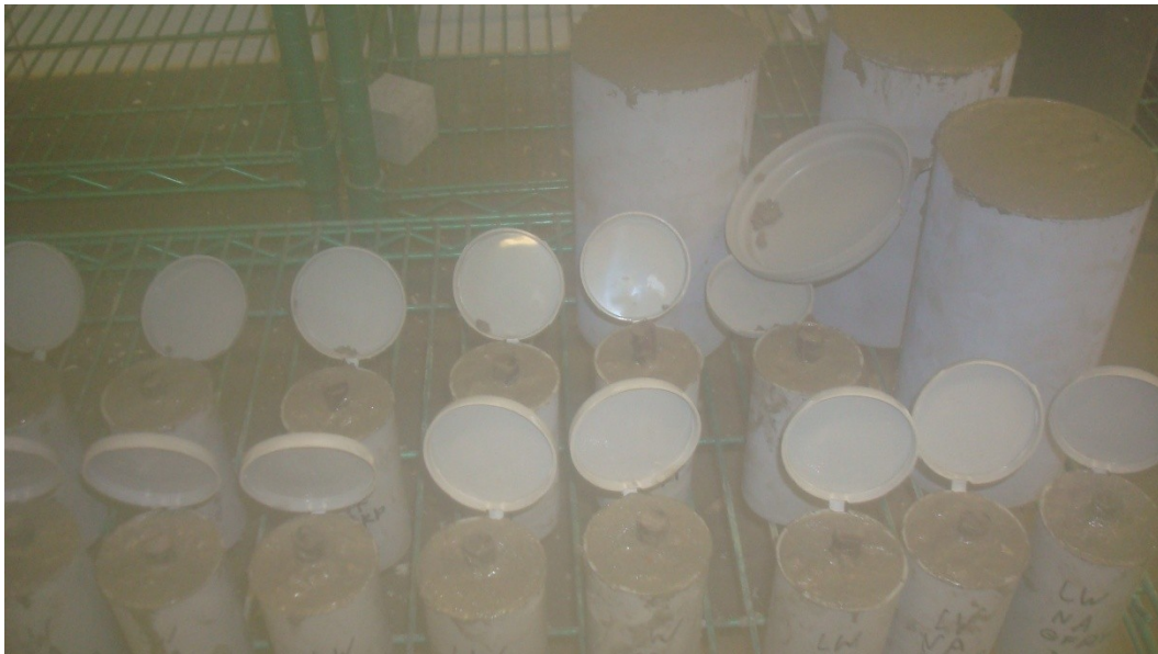
Figure 3-5 Concrete in the curing chamber
