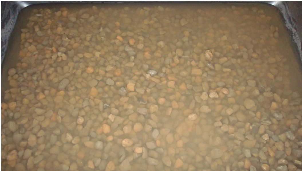
Figure 3-3 Lightweight Aggregates Soaking
