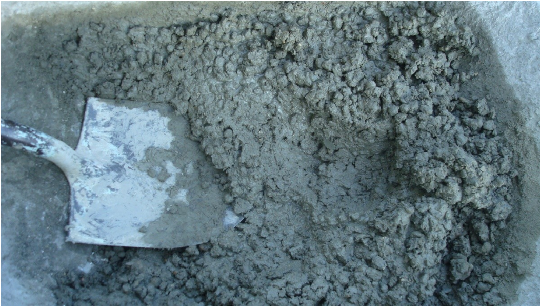
Figure 3-4 Fresh lightweight concrete mix
