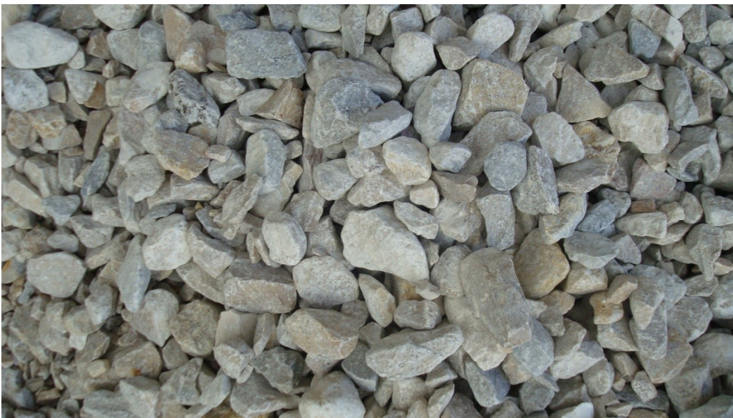
Figure 3-2 Normalweight Aggregates from UTA stock, sieved to 3/4" maximum size
