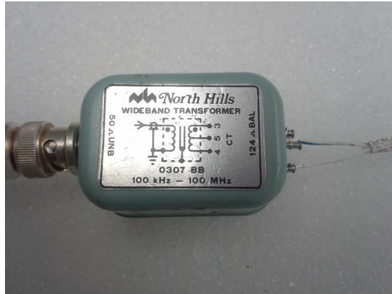
Figure 4-12 Close-up of balun nomenclature plate
