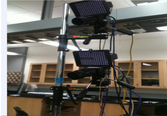
Figure 2-2: Optimized Position of two cameras for 3D tracking of targets
