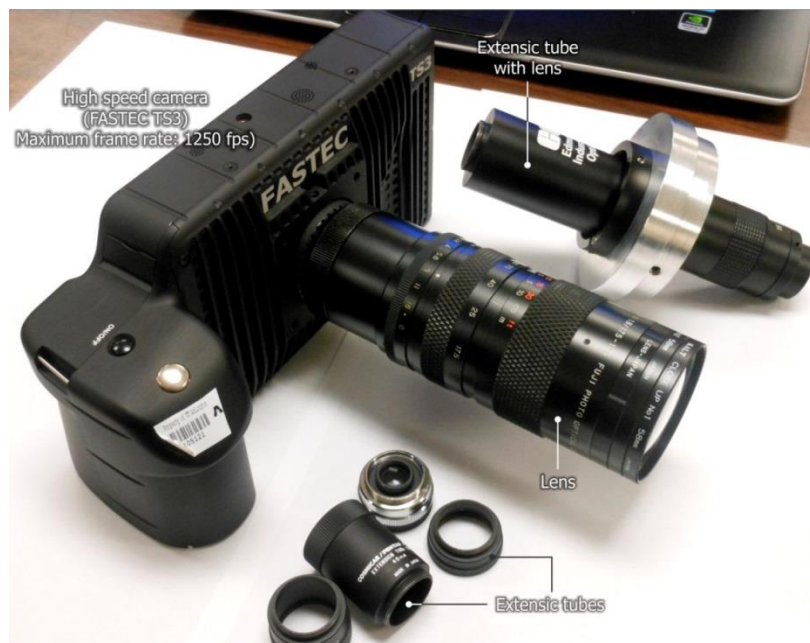
Figure 2.12 The high speed camera (FASTEC, TS3), lenses and extensic tubes used for the test
