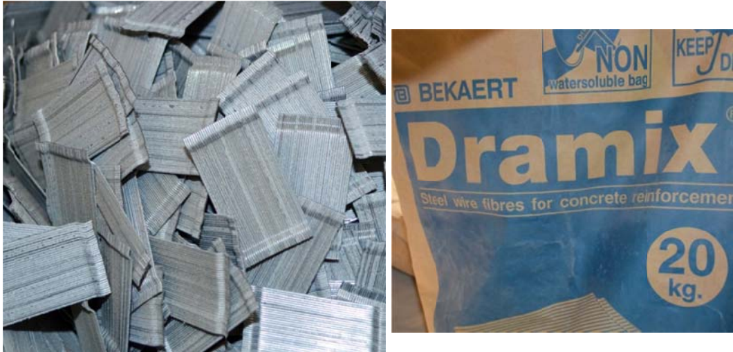
Figure 2-2 Photograph of Typical Steel Fibers (RC-65/35-BN) used
