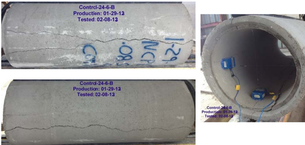
Figure B-128 Crack propagation for RCP-24-6-B
