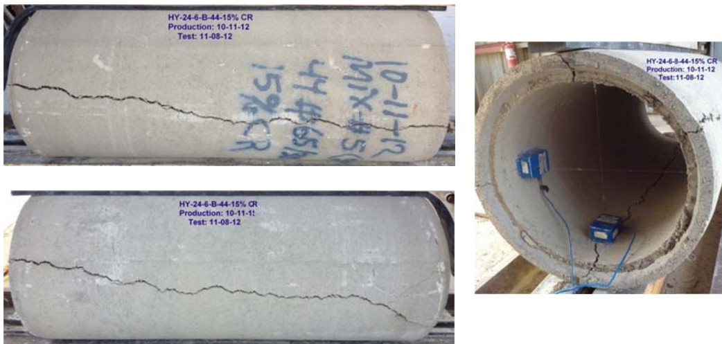
Figure B-99 Crack propagation for HYCP-24-6-B-44lbs steel-15%rubber
