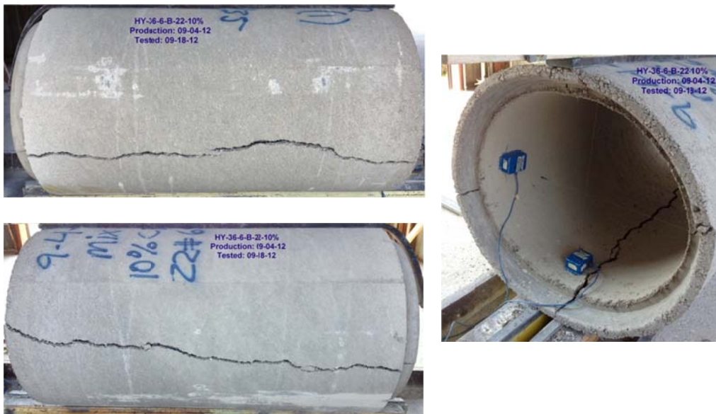
Figure B-70 Crack propagation for HYCP-36-6-B-22-10%rubber
