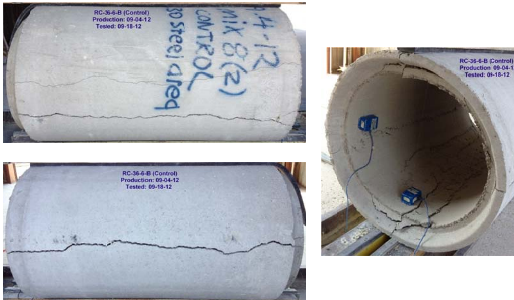
Figure B-68 Crack propagation for RCP-36-6-B
