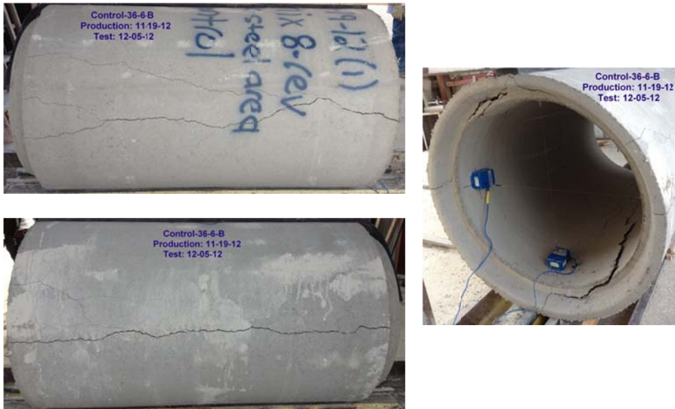
Figure B-118 Crack propagation for RCP-36-6-B
