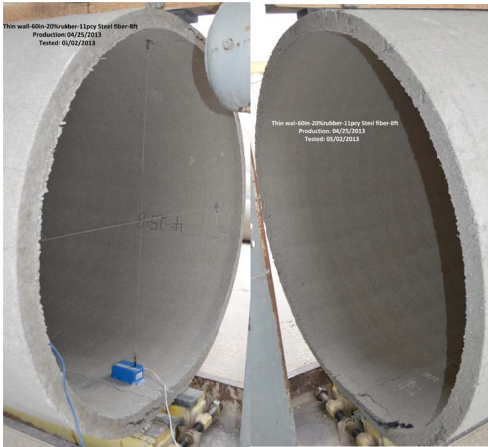
Figure B-149 Crack propagation for Thin wall-60"-11PCY SF-20% rubber-8ft
