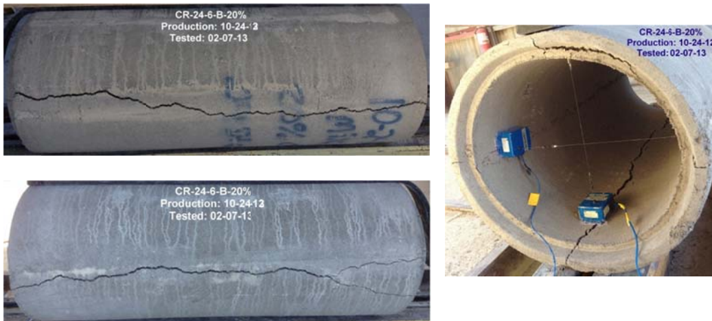
Figure B-112 Crack propagation for CRCP-24-6-B-20%rubber
