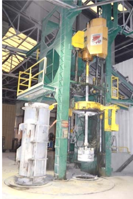
Figure 1-2 Photograph of Packerhead Machine
