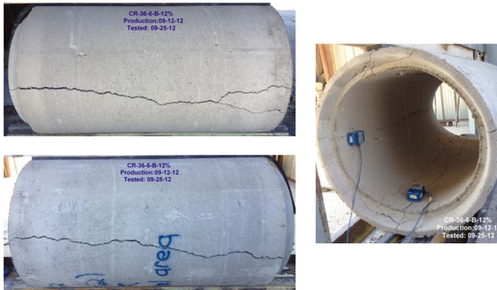
Figure B-80 Crack propagation for CRCP-36-6-B-12%rubber
