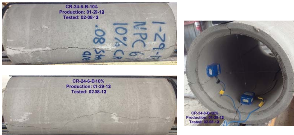
Figure B-134 Crack propagation for CRCP-24-6-10%rubber
