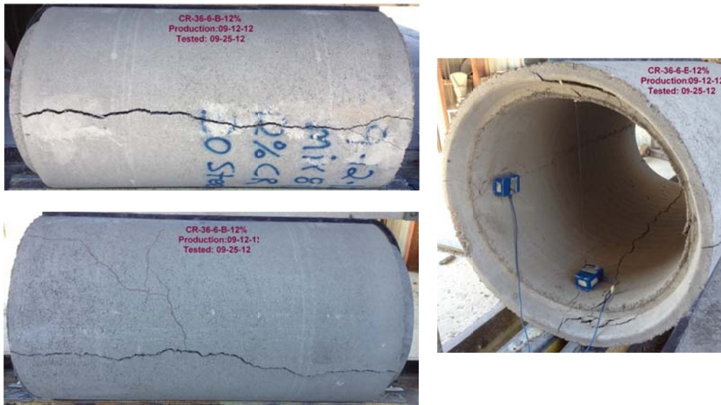
Figure B-78 Crack propagation for CRCP-36-6-B-12%rubber
