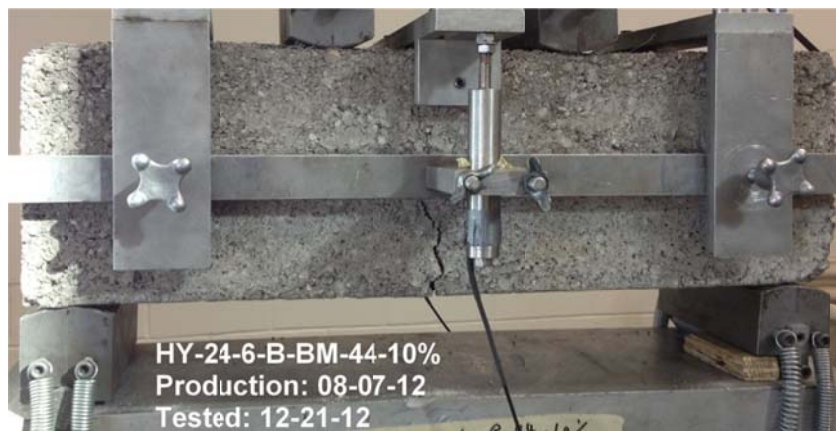
Figure C-14 Photograph of HY-24-6-BM-44lbs-10%
