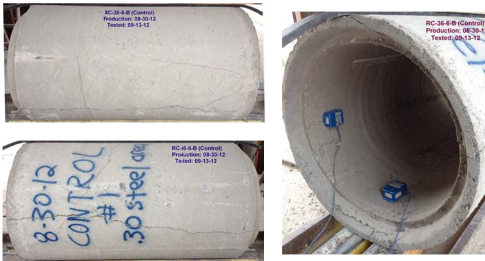
Figure B-54 Crack propagation for RCP-36-6-B
