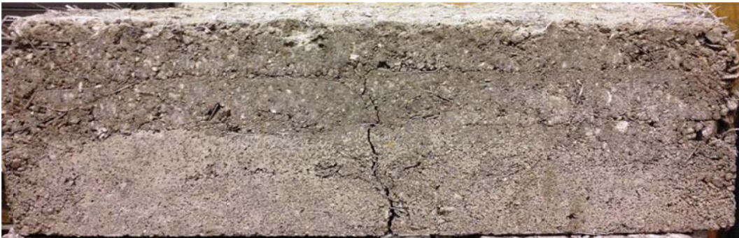
Figure C-90 Photograph of HY-44lbs steel-5lbs synth-3%
