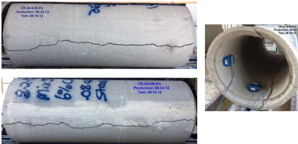
Figure B-14 Crack propagation for CRCP-24-6-B-6%rubber
