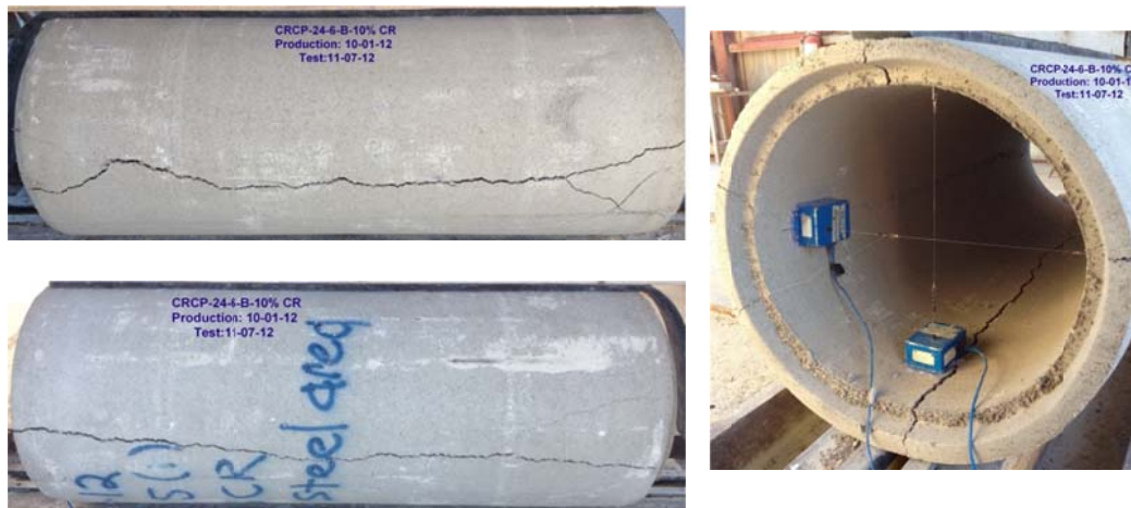
Figure B-90 Crack propagation for CRCP-24-6-B-10%rubber
