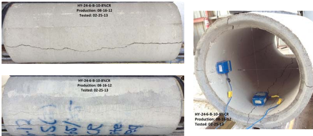
Figure B-44 Crack propagation for HYRCP-24-6-B-10lbs steel-8% rubber
