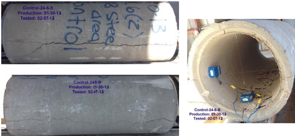
Figure B-141 Crack propagation for RCP-24-6-B
