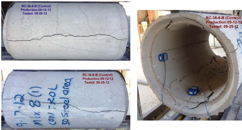
Figure B-72 Crack propagation for RCP-36-6-B
