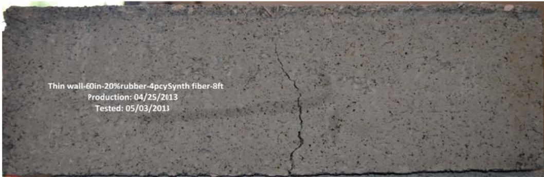
Figure C-108 Photograph of Thin wall-60in-4PCY Synth-20% rubber-8ft
