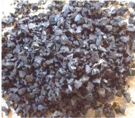
Figure 2-1 Photograph of Typical Crumb Rubber Used
