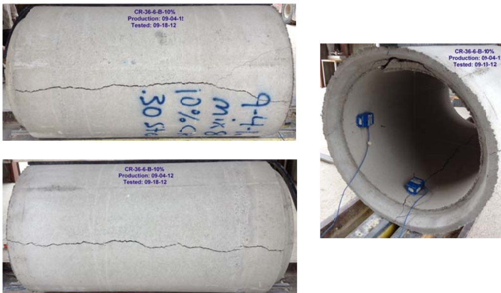
Figure B-60 Crack propagation for CRCP-36-6-B-10%rubber
