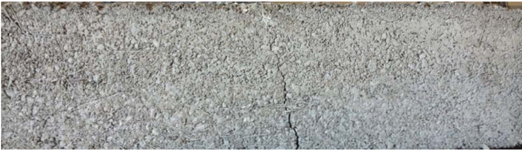
Figure C-78 Photograph of HY-36-6-B-BM-8% synth-20% rubber
