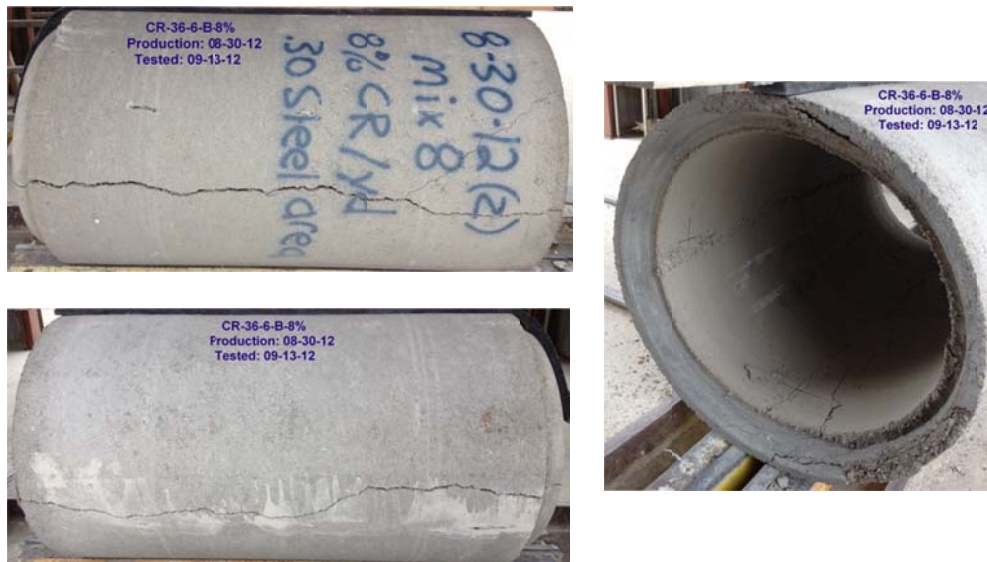
Figure B-52 Crack propagation for CRCP-36-6-8%rubber
