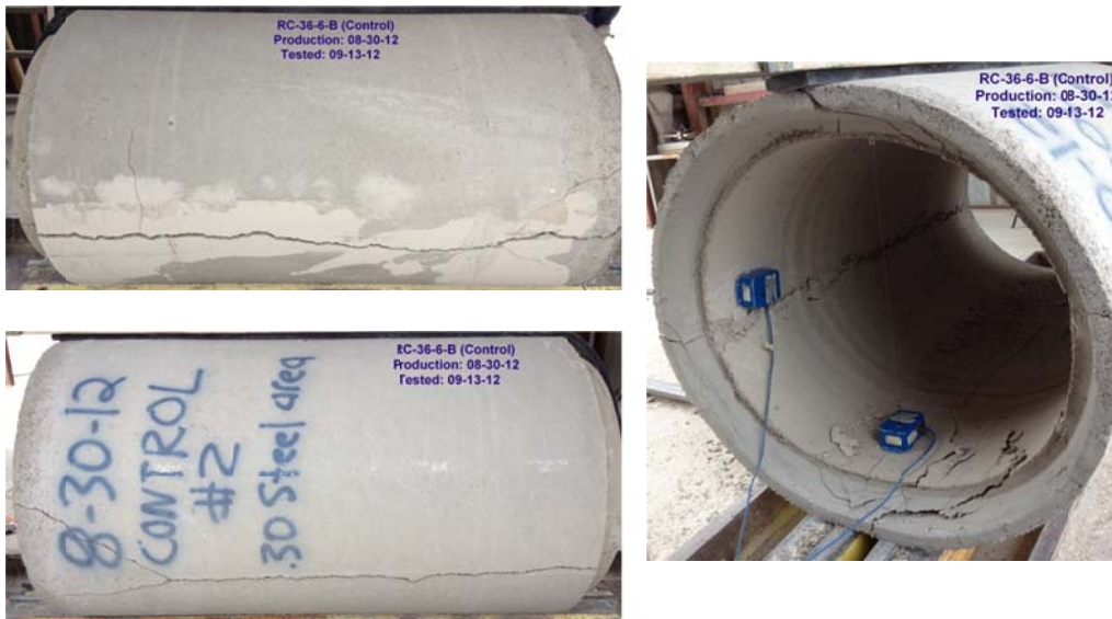
Figure B-56 Crack propagation for RCP-36-6-B
