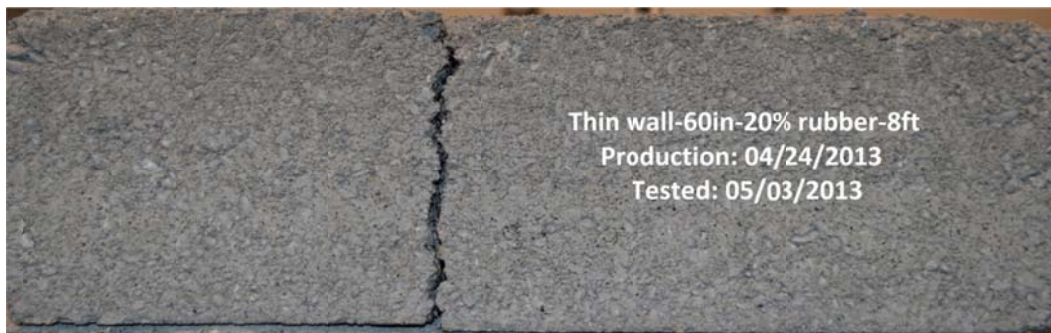
Figure C-100 Photograph of Thin wall-60in-20% rubber-8ft
