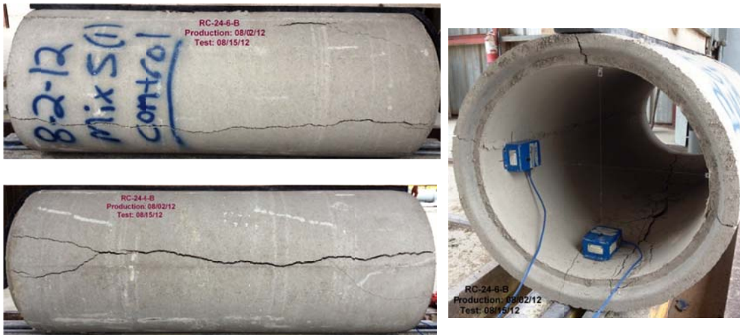
Figure B-24 Crack propagation for RCP-24-6-B
