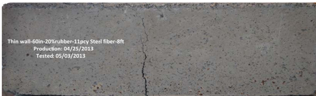
Figure C-104 Photograph of Thin wall-60in-11PCY SF-20% rubber-8ft
