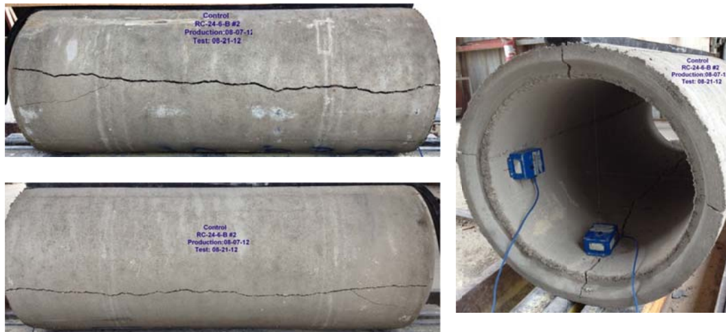
Figure B-28 Crack propagation for RCP-24-6-B
