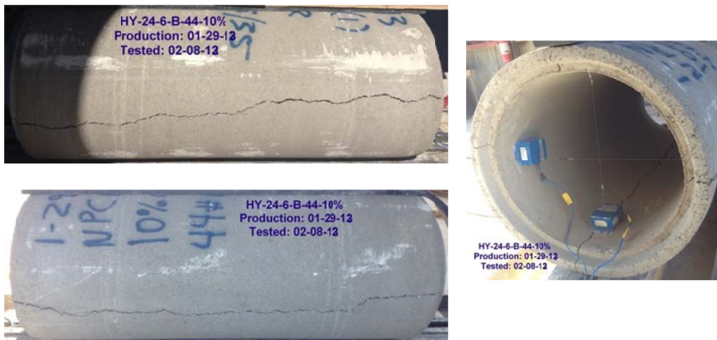
Figure B-124 Crack propagation for HYCP-24-6-B-44lbs steel-10%rubber
