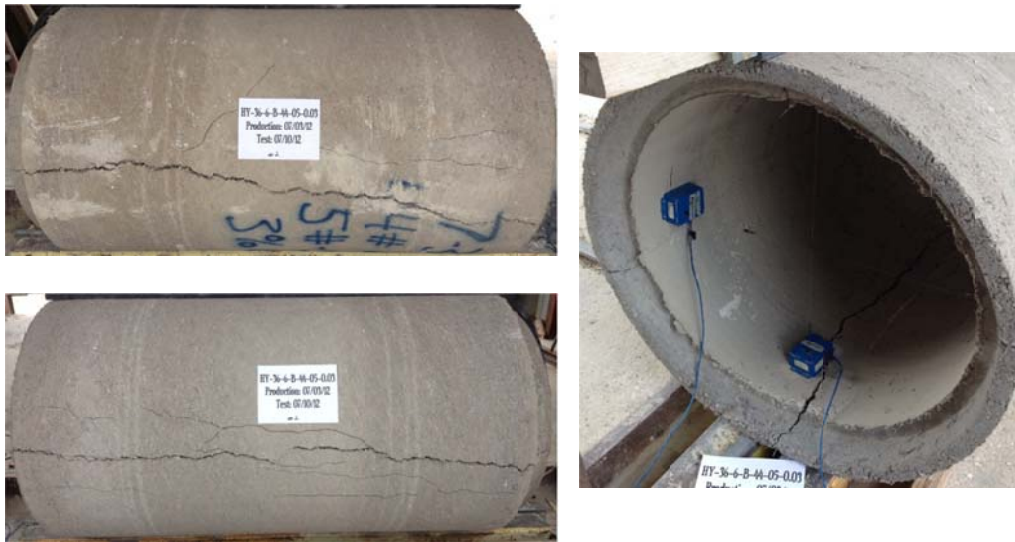
Figure B-6 Crack propagation for HYCP-36-6-B-44lbs steel-3% rubber-5lbs synth
