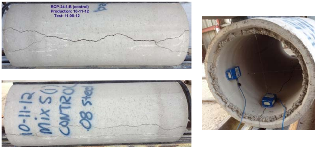
Figure B-103 Crack propagation for RCP-24-6-B
