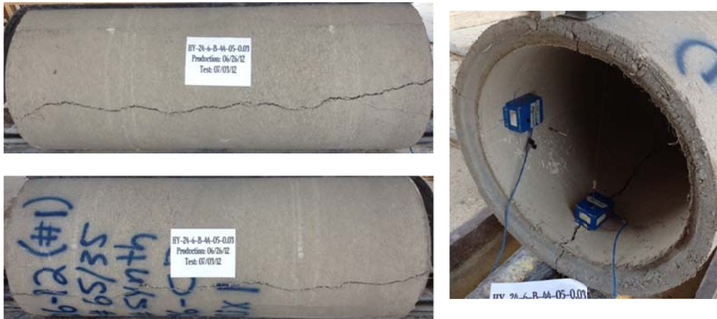
Figure B-4 Crack propagation for HYCP-24-6-B-44lbs steel-3% rubber-5lbs synth
