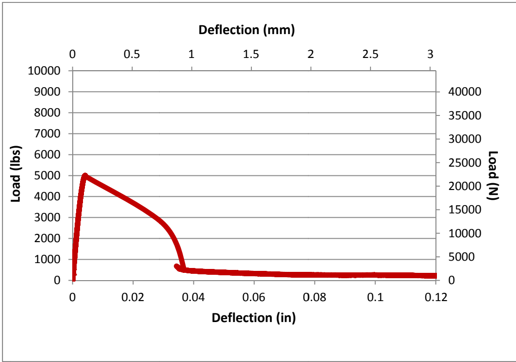
Figure C-5 Load-Deflection Plot for CR-24-6-BM-8%
