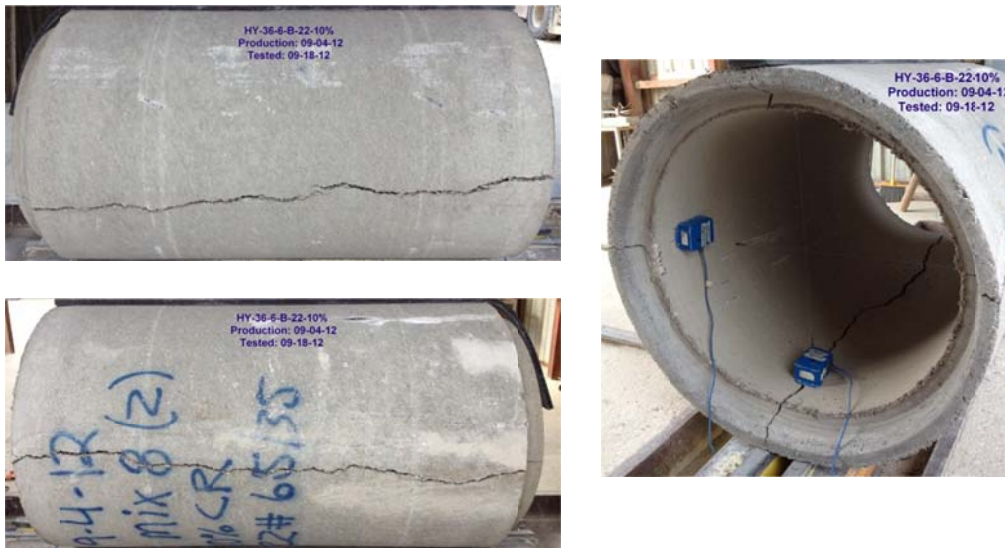
Figure B-62 Crack propagation for HYCP-36-6-B-22-10%rubber
