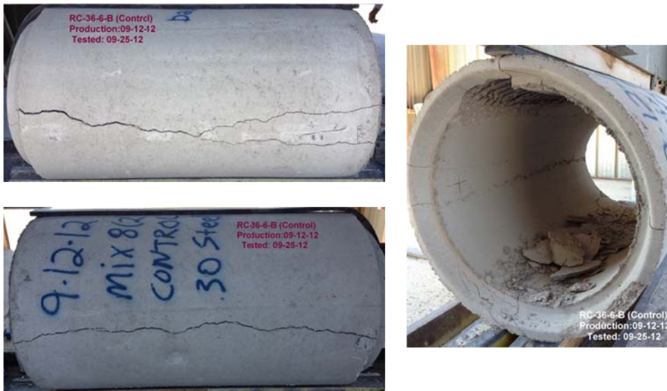
Figure B-76 Crack propagation for RCP-36-6-B
