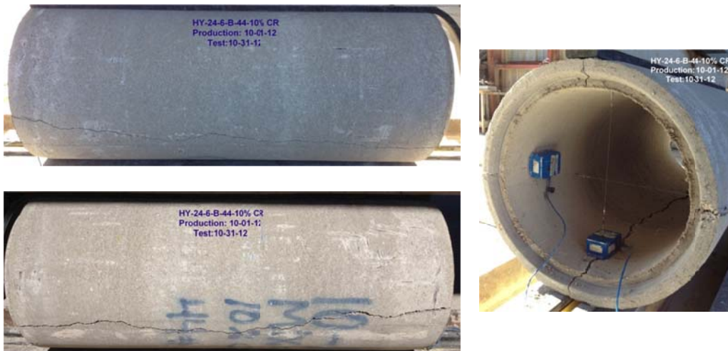
Figure B-82 Crack propagation for HYCP-24-6-B-44lbs steel-10%rubber
