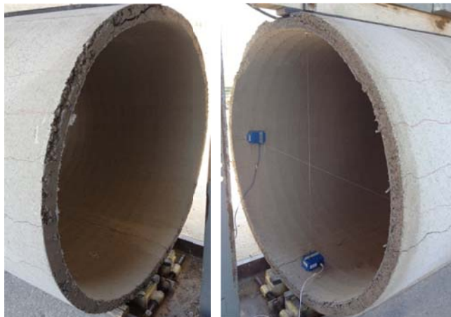
Figure B-143 Crack propagation for Thin wall-60-8-13%rubber
