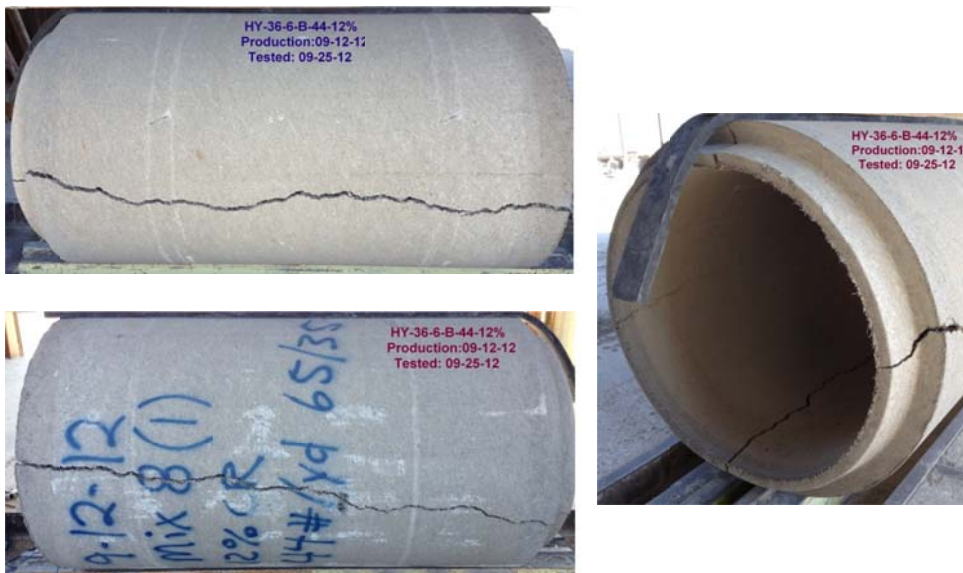
Figure B-74 Crack propagation for HYCP-36-6-B-44lbs steel-12%rubber
