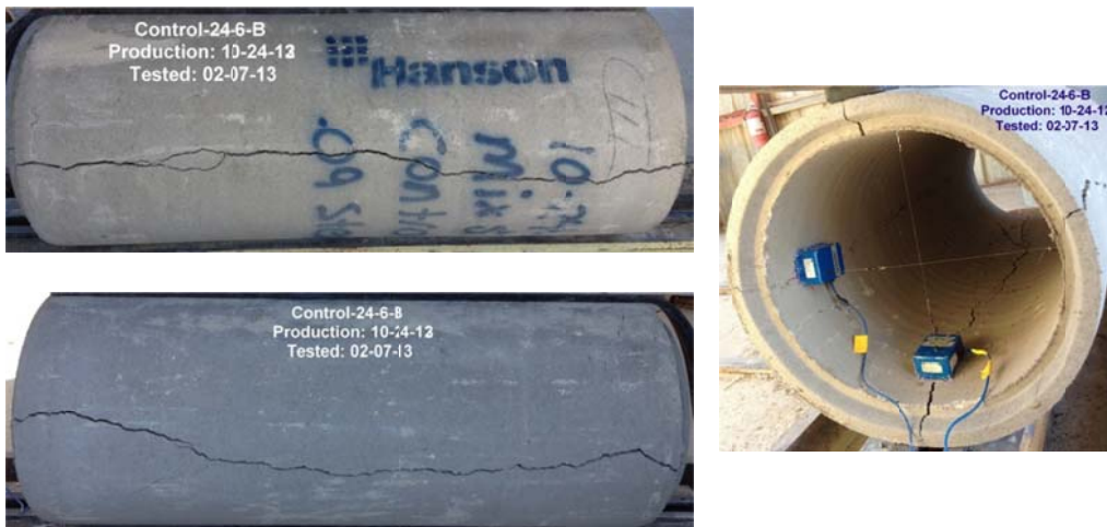
Figure B-114 Crack propagation for RCP-24-6-B
