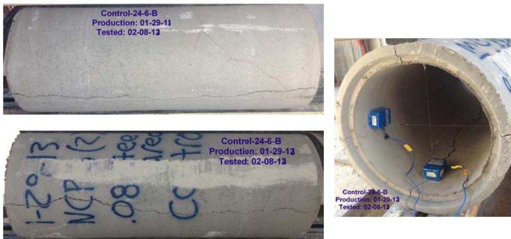
Figure B-132 Crack propagation for RCP-24-6-B
