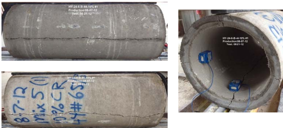
Figure B-34 Crack propagation for HYCP-24-6-B-44lbs steel-10%rubber
