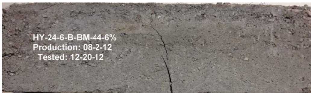
Figure C-12 Photograph of Crack for HY-24-6-BM-44lbs-6%
