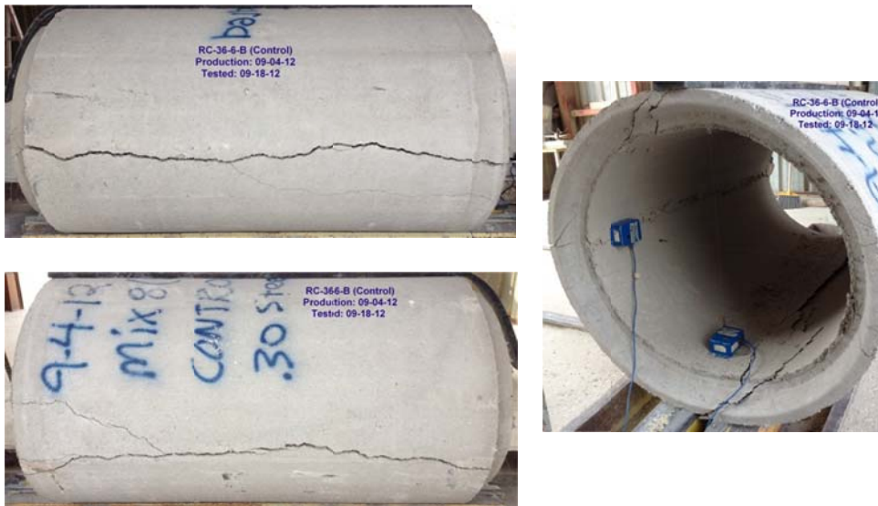
Figure B-64 Crack propagation for RCP-36-6-B
