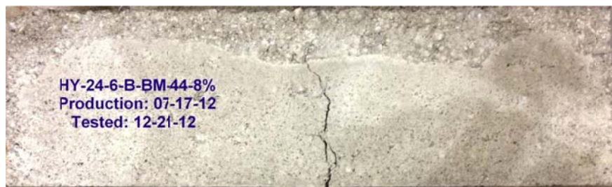
Figure C-2 Photograph of Crack for HY-24-6-BM-44lbs-8%
