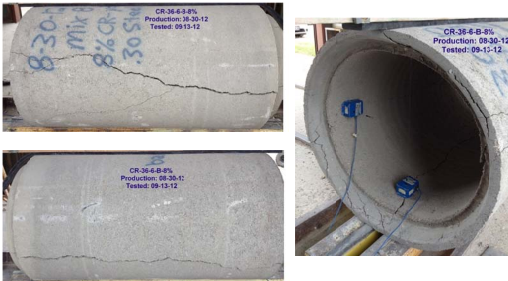
Figure B-48 Crack propagation for CRCP-36-6-8%rubber
