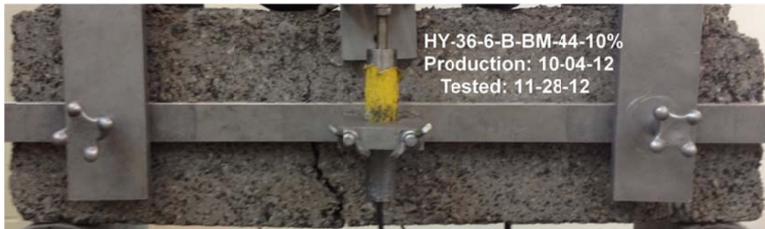
Figure C-52 Photograph of HY-36-BM-44lbs-10%
