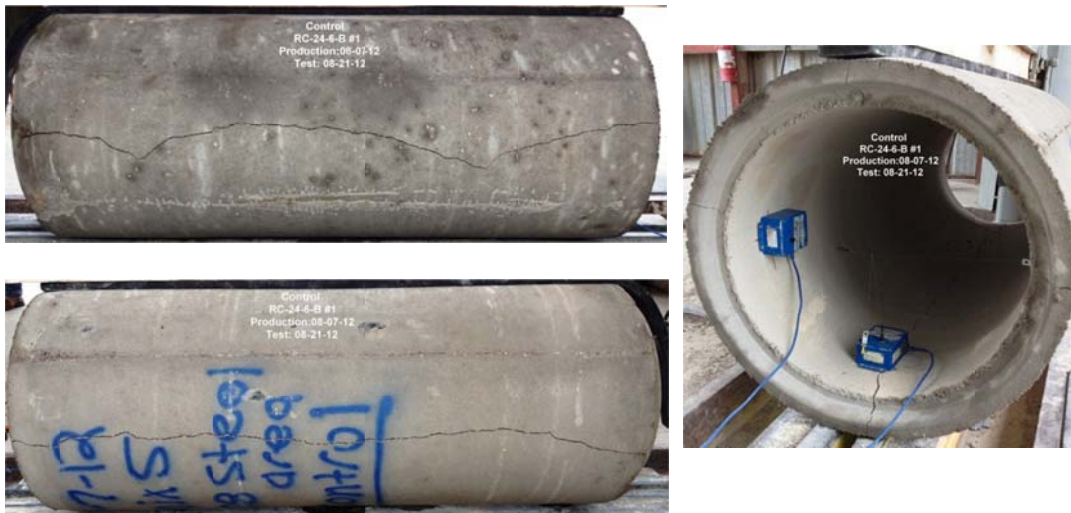
Figure B-26 Crack propagation for RCP-24-6-B
