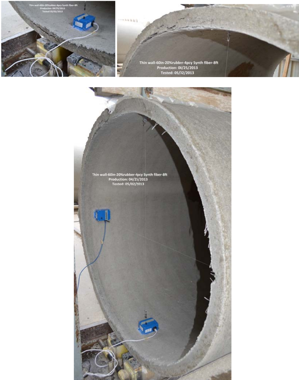
Figure B-151 Crack propagation for Thin wall-60"-4PCY Synth-20% rubber-8ft
