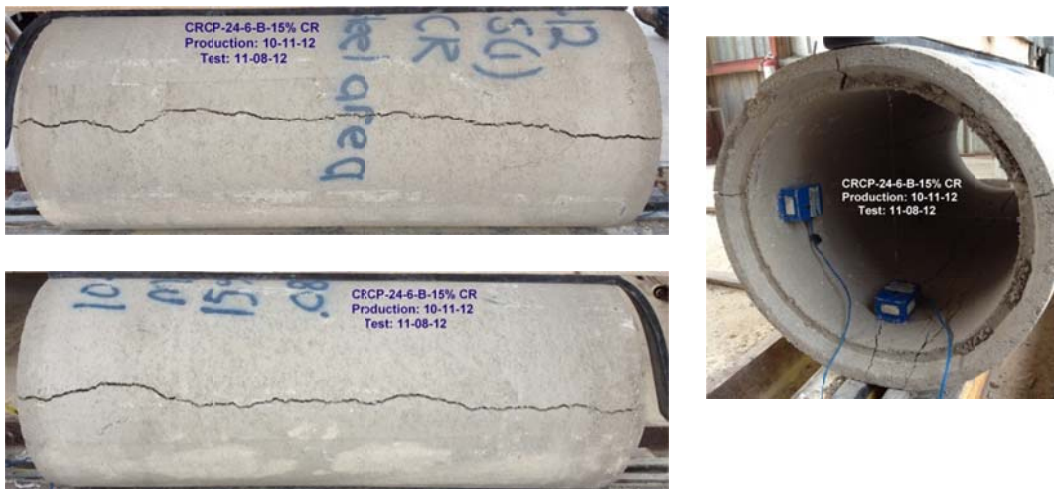
Figure B-105 Crack propagation for CRCP-24-6-B-15%rubber
