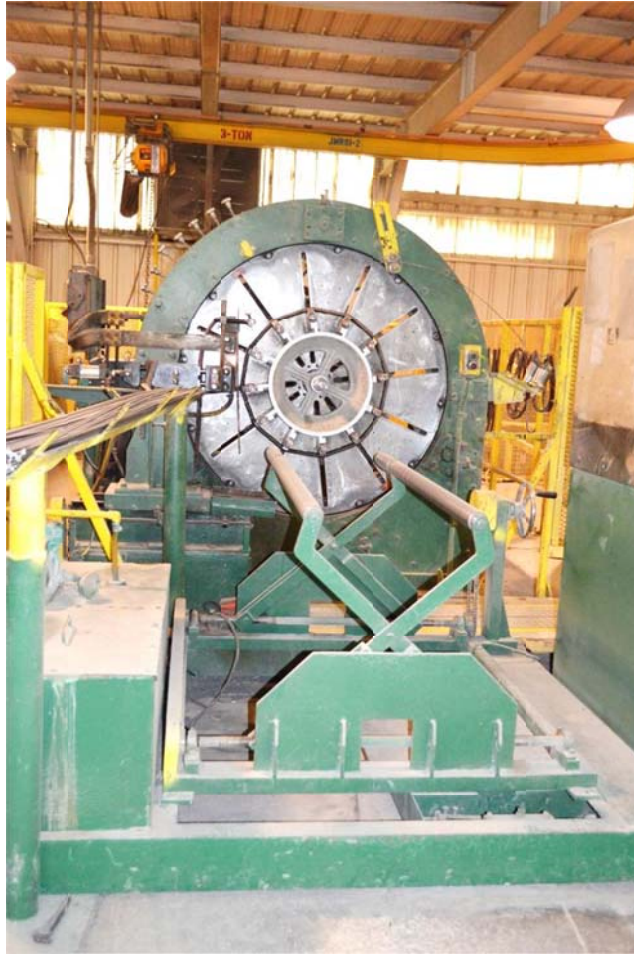
Figure 1-1 Photograph of Steel cage machine at Hanson facility in Grand prairie, TX
