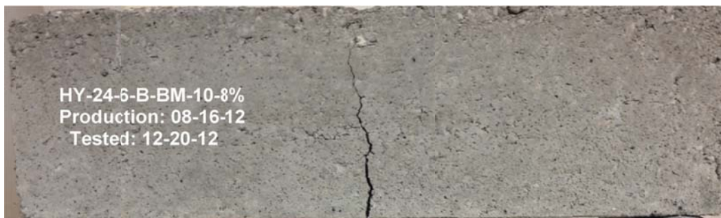
Figure C-22 Photograph of HY-24-6-BM-10lbs-8%
