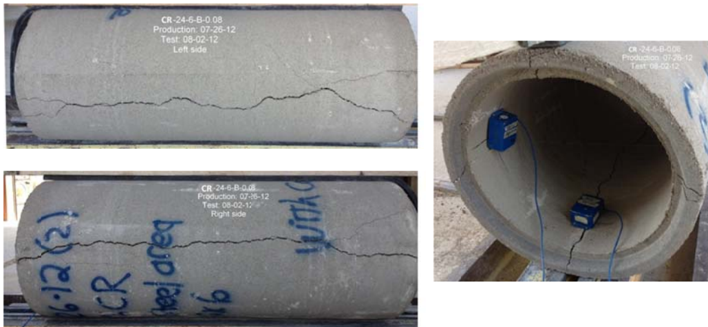
Figure B-10 Crack propagation for CRCP-24-6-B-8%rubber
