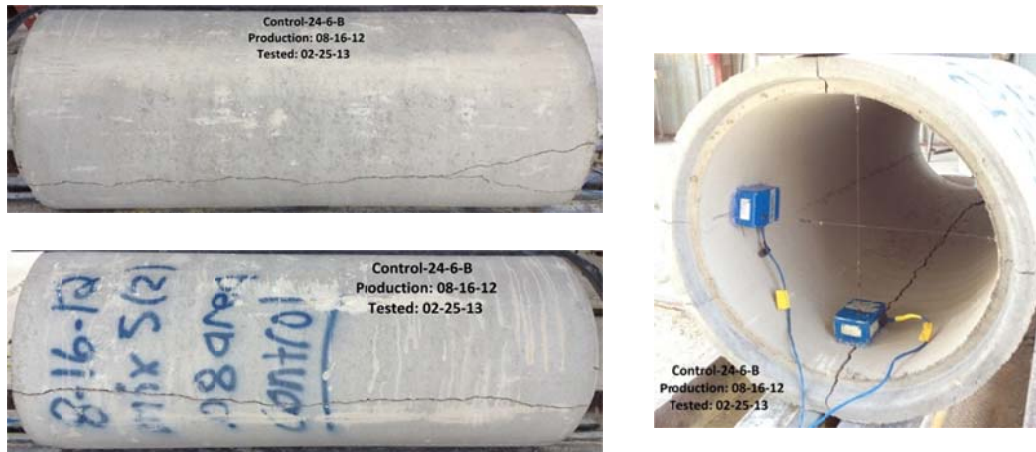
Figure B-46 Crack propagation for RCP-24-6-B
