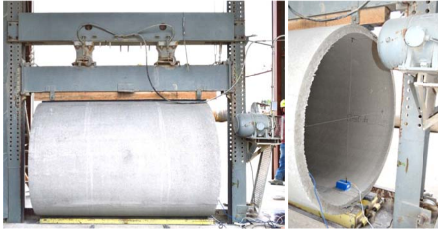
Figure 3-1 Photograph of D-Load rack at Hanson facility
