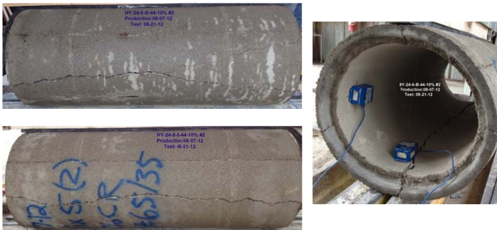
Figure B-36 Crack propagation for HYCP-24-6-B-44lbs steel-10%rubber
