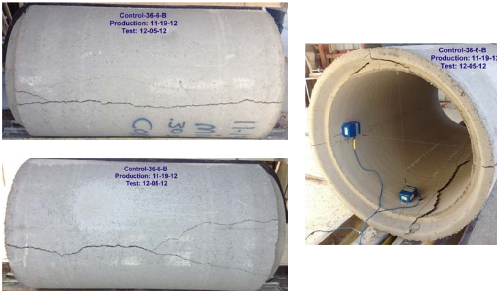
Figure B-116 Crack propagation for RCP-36-6-B
