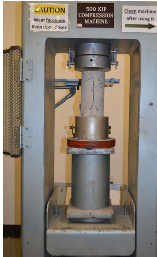
Figure 4-5 Photograph of Compressive Cylinder Testing Machine at CELB
