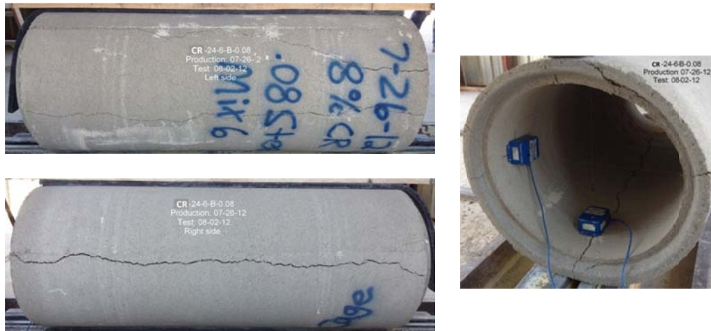
Figure B-12 Crack propagation for CRCP-24-6-B-8%rubber
