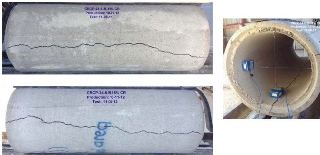
Figure B-95 Crack propagation for CRCP-24-6-B-15%rubber
