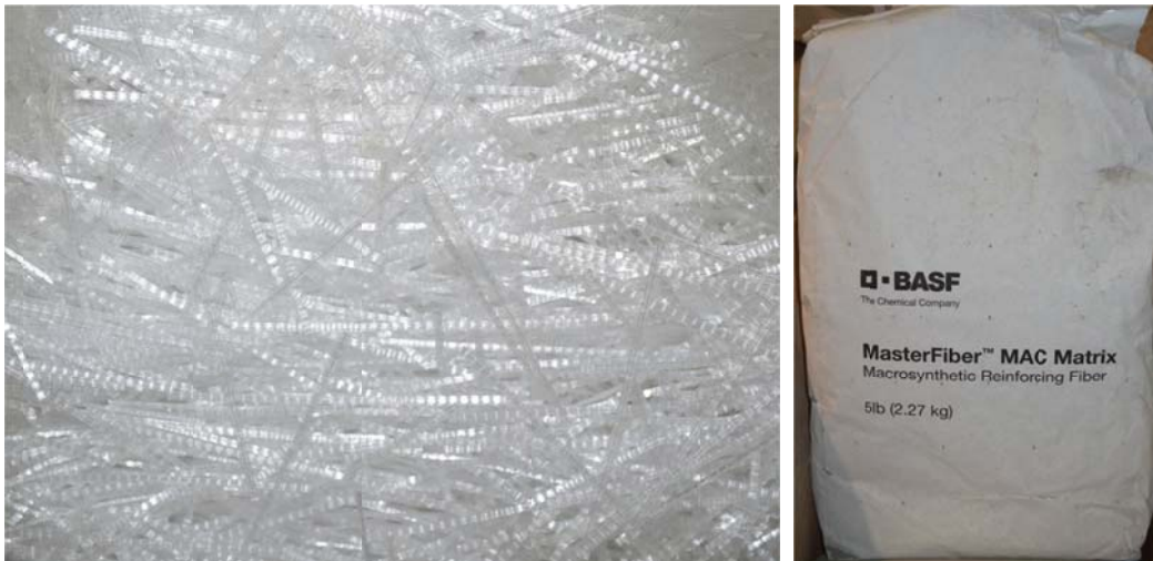
Figure 2-3 Photograph of Macrosynthetic fibers used in this study
