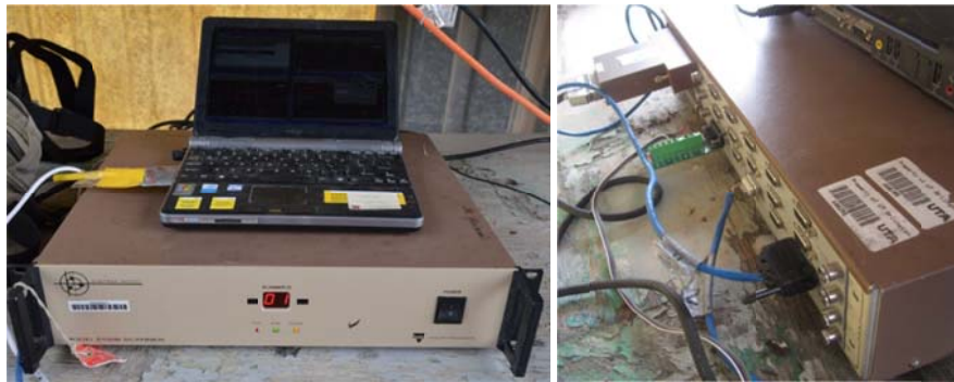
Figure 3-2 Data acquisition unit (Vishay scanner)
