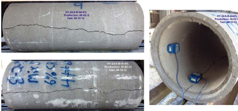
Figure B-18 Crack propagation for HYCP-24-6-B-44lbs steel-6%rubber
