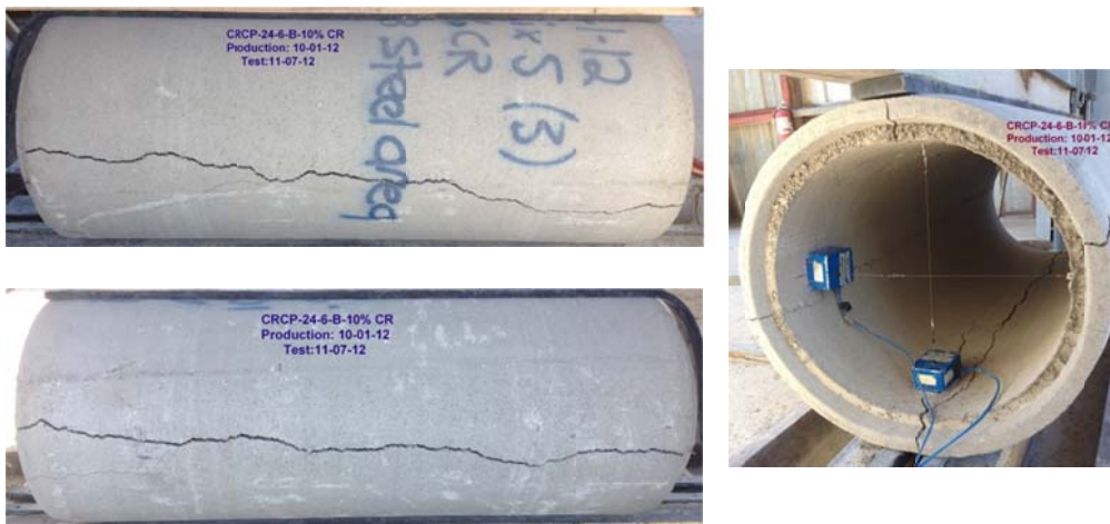
Figure B-84 Crack propagation for CRCP-24-6-B-10%rubber
