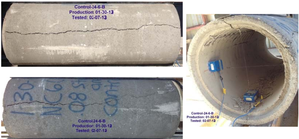
Figure B-136 Crack propagation for RCP-24-6-B
