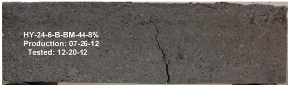
Figure C-6 Photograph of Crack for HY-24-6-BM-44lbs-8%
