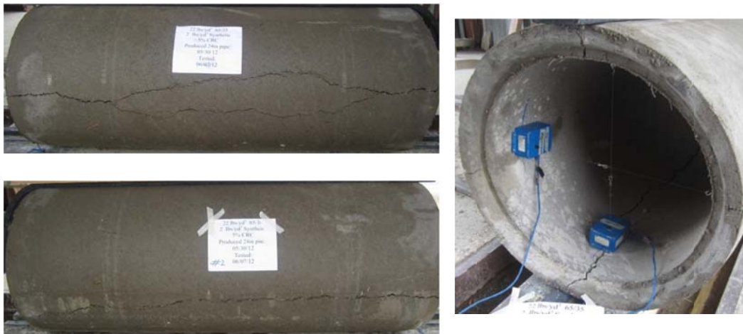
Figure B-2 Crack propagation for HYCP-24-6-B-22lbs steel-5% rubber-2%synth
