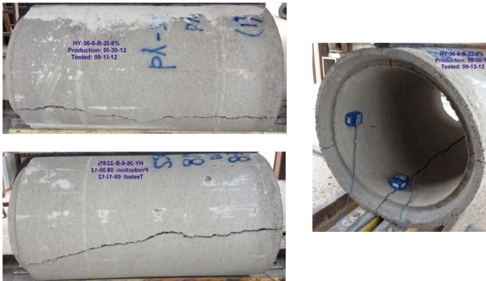
Figure B-50 Crack propagation for HYCP-36-6-22lbs steel-8%rubber
