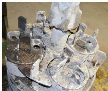
Figure 1-3 Photograph of Roller heads in Packerhead Machine
