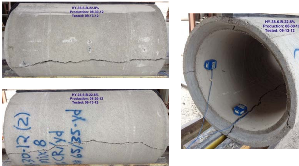
Figure B-58 Crack propagation for HYCP-36-6-22-8% rubber
