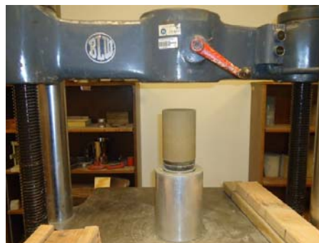
Figure 3.5 Gyratory Compactor Machine, (b) Soil sample after extraction
