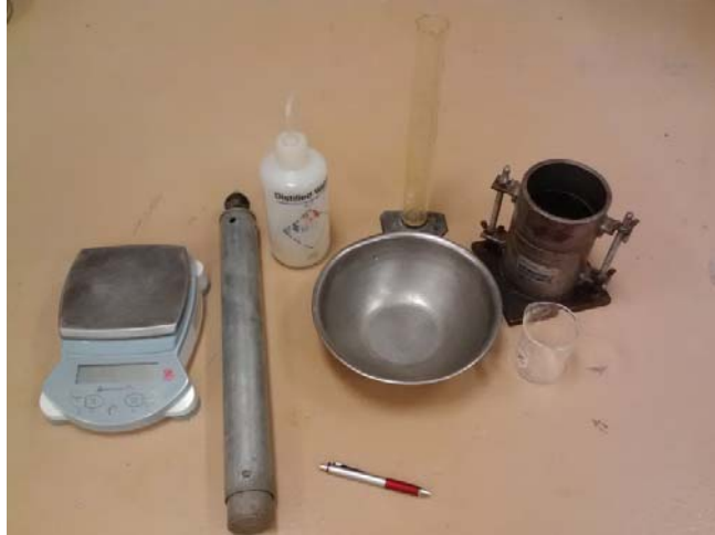
Figure 3.3 Standard proctor compaction test apparatus
