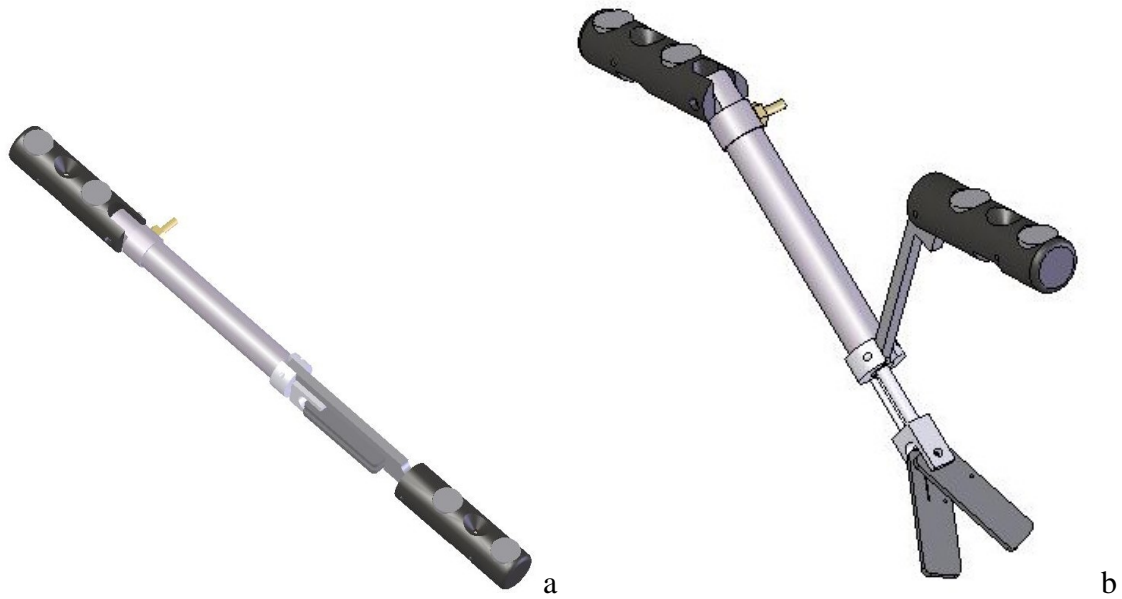
Figure 15. Paddle retractor revision c. For insertion (a), the tool folds to fit through the trocar. After insertion, the tool unfolds (b) and is ready for use.
