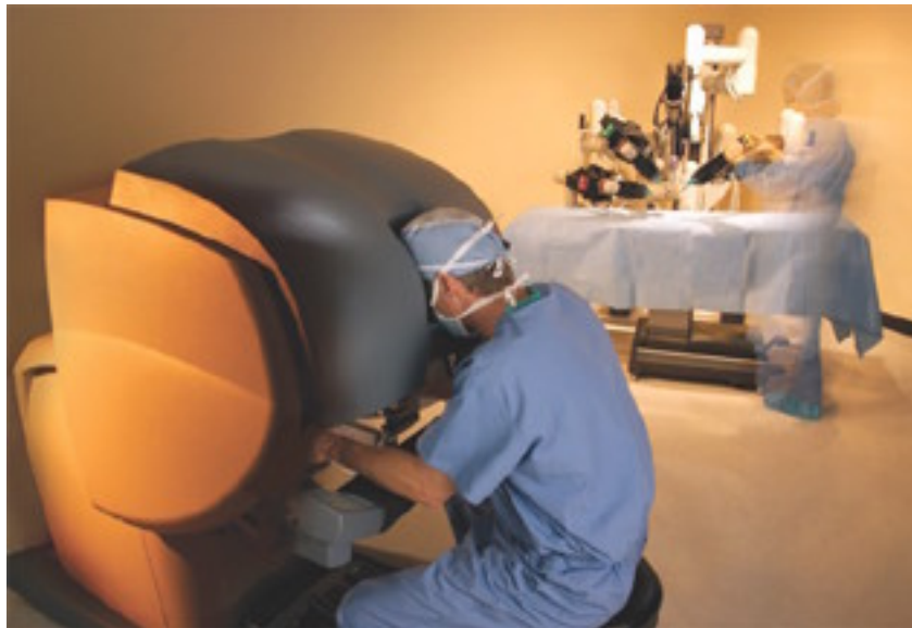
Figure 3. The daVinci surgical system. The surgeon sits at a console away from the surgical table and controls the motions of the robot.
